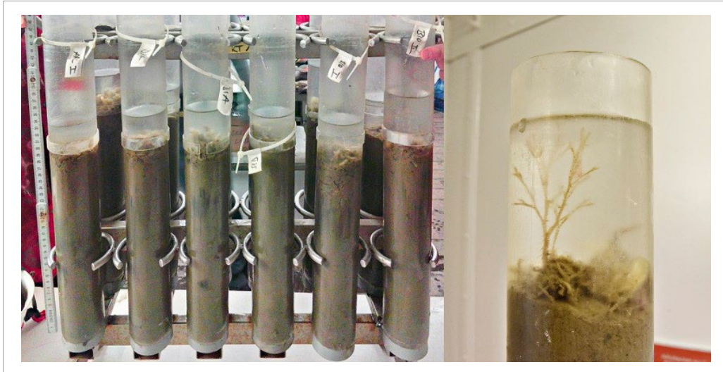
Fig. 3.3: Example of photo-documented MUC tubes retrieved at station PS141_54-6 in Vincennes Bay (121 m water depth). Note the macro-benthos in the upper part of the sediment.
