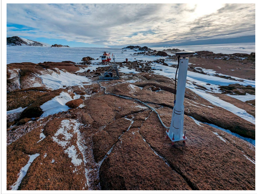
Fig. 6.2.6: GNSS monument and antenna at WABF/Watson Bluff, looking true west
