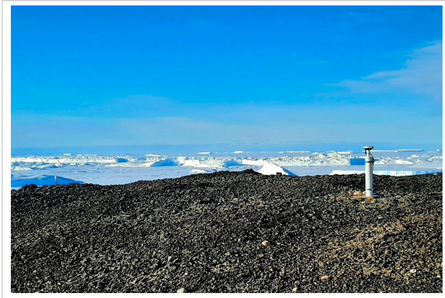
Fig. 6.2.4: GNSS pillar and antenna at GAP1/Gaussberg, looking north. To the left, just at the edge of the rim, the Iridium antenna can be seen (mounted at top of the frame, cf. Fig. 6.2.5).
