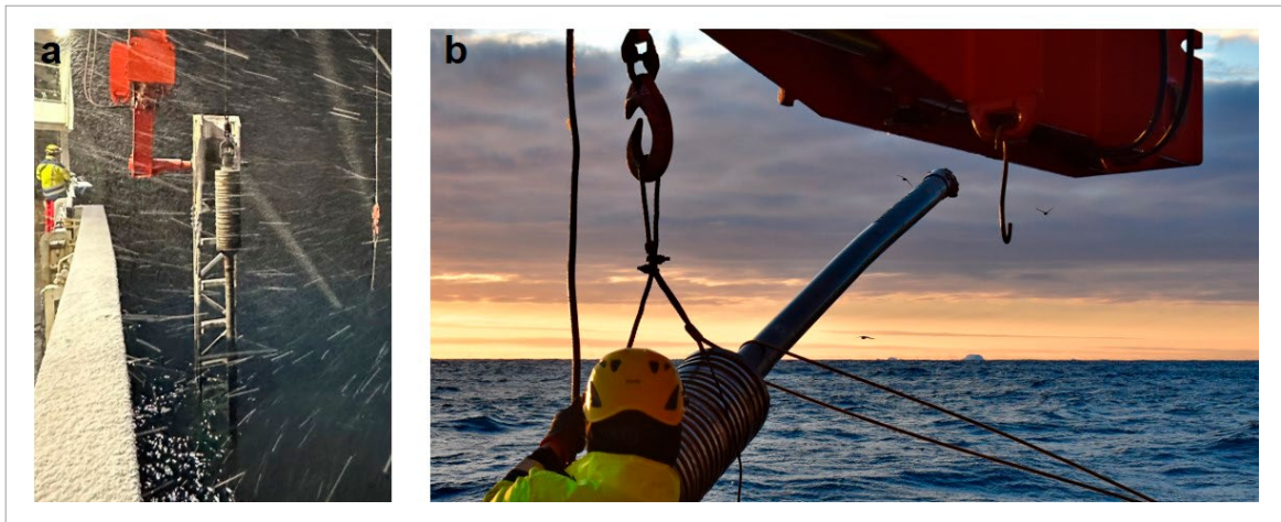
Fig. 3.4: Deployment of the gravity corer a) with and b) without a core handling rack during Polarstern expedition PS141
