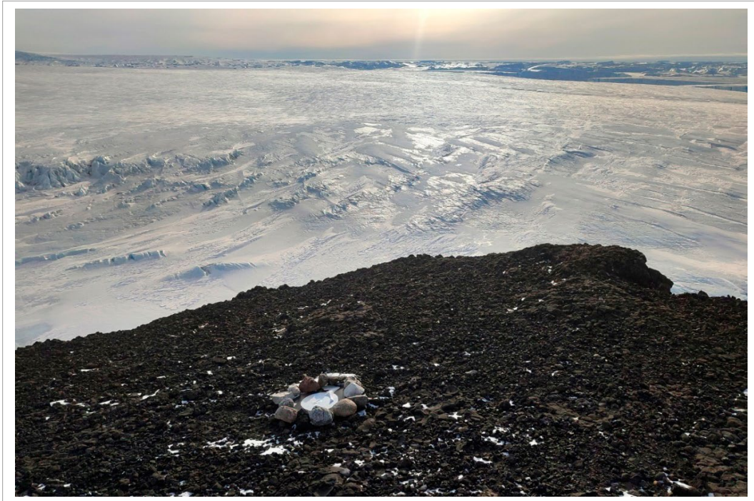
Fig. 6.2.21: Temporarily established ground control point GCP1 (close to Kap Lewald)
