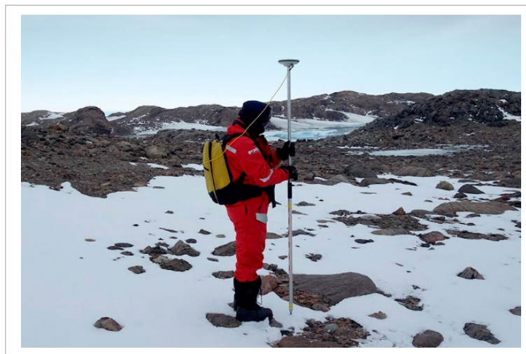
Fig. 6.2.24: GNSS positioning to document heights of emergent marine shorelines, Thomas I.
