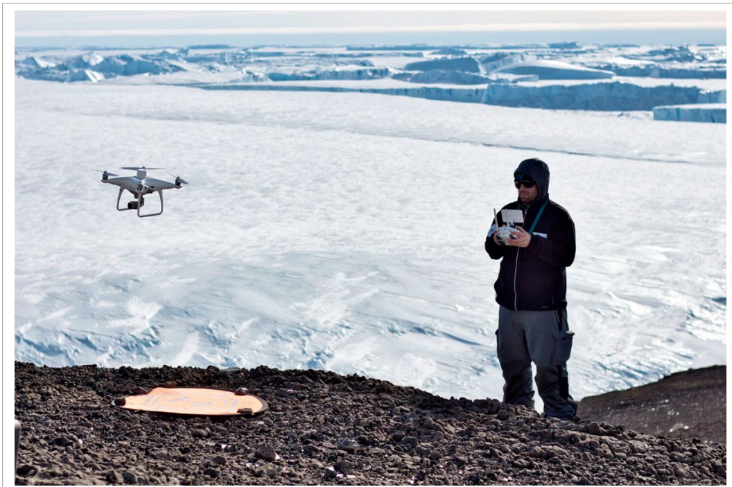
Fig. 6.2.20: UAV DJI Phantom 4 RTK used as the main platform for the acquisition of aerial images of the different study areas. This photo shows the take-off and landing area, supported by the special landing pad, used as a basis for the flight over the glacier.
