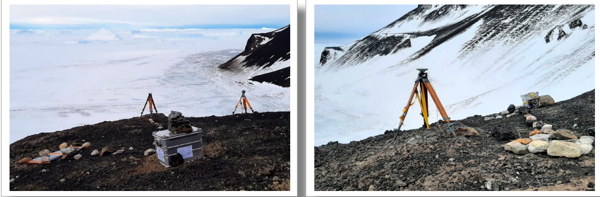
Fig. 6.2.17: Set-up of the GNSS site GOCE, looking at the northern bay of Gaussberg to infer measurements of the local sea level by GNSS reflectometry. Left: Initial set-up (28.02.- 03.03.2024). Right to the GNSS antenna the tripod with the time-laps camera was installed (see also Fig. 6.2.20). At the right margin in the middleground: Nordkap. Right: Second set-up (11.-15.03.2024)
