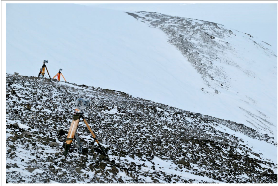
Fig. 6.2.19: System of four cameras installed at the edge of the camp plateau for 2D and 3D monitoring of the glacier west of Gaussberg
