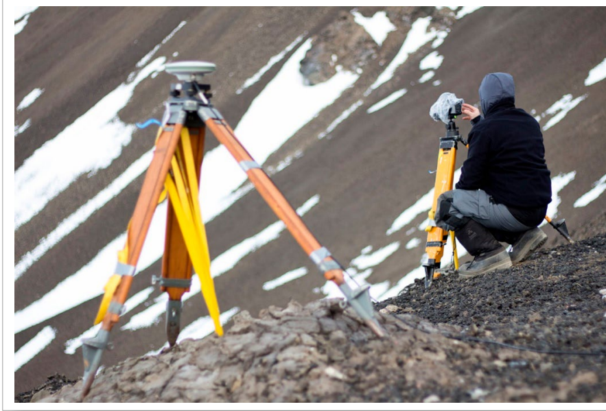
Fig. 6.2.18: Camera installed at the right tripod, pointing towards the northern bay of Gaussberg for 2D monitoring of ocean tides. At the left tripod the antenna of the temporary GNSS station GOCE is mounted (see also Fig. 6.2.19).
