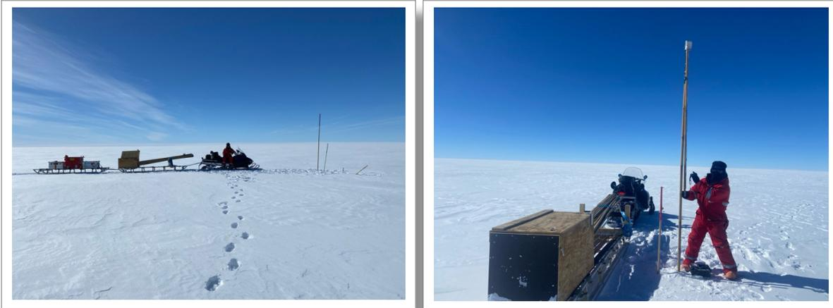
*Fig. 4.8.2: Accumulation stake measurements: Left (a): Setup of snowmachine train. Right (b): measuring the height of a bamboo stake higher than 2 m with an extension and a wireline device, which automatically records GPS positions.*
