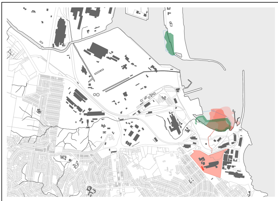
Figure 5. Diagram indicating the intersections between the seabed chemical contaminants from the copper refinery and the dredging and emplacement works.
