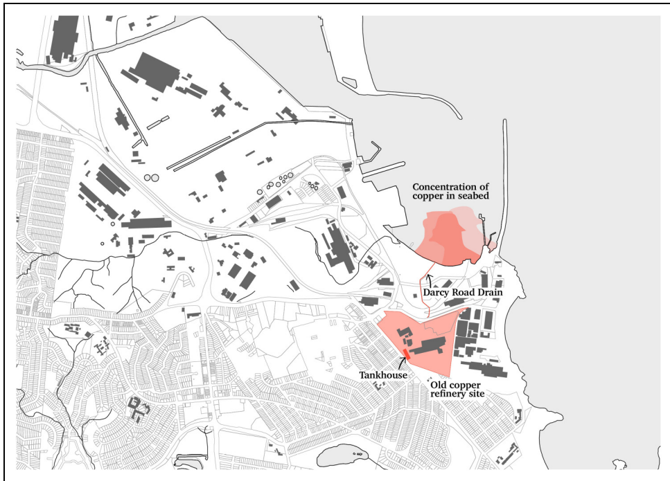
Figure 2. Diagram indicating the location of the old copper refinery, contaminant flows down Darcy Road Drain, and harbour seabed sediments containing high levels of copper at the outlet of Darcy Road Drain, the latter data loosely adapted from Jones et al. (2019).
