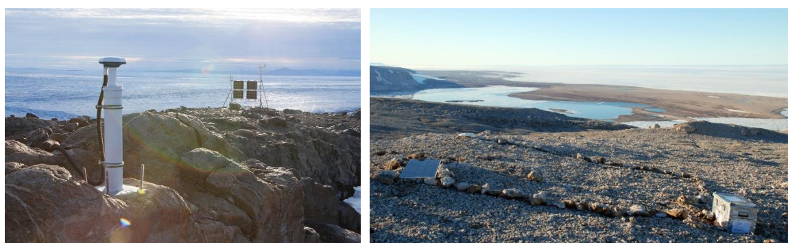
Fig. 5.3: GNSS installations at Lambert Land West (LAP1, 2022, left) and Holm Land (HOLM, 2008, right). At LAP1 the GNSS antenna is mounted on top of a special pillar fixed to bedrock. Receiver, batteries and further equipment are stored in two Zarges aluminium boxes (mounted at the structure in the background), while four solar panels and a wind generator are used to recharge the batteries. At HOLM the GNSS antenna will be mounted at a special bolt which is fixed in bedrock ("forced centering"). Receiver, battery and further equipment are stored in the Zarges aluminium box, while a solar panel is used to recharge the battery.
