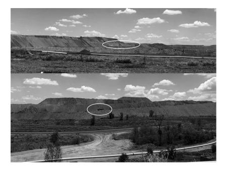
**Note:** Above: a vehicle driving up the waste rock piles has a cloud of dust behind it. Below: a water vehicle is spraying the waste rock road to minimise dust.
