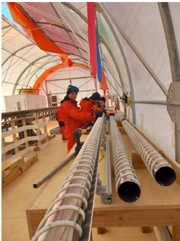
Fig. 5.1.1: Alignment of the core extraction table and electrical wiring of the FED (fluid extraction device).
