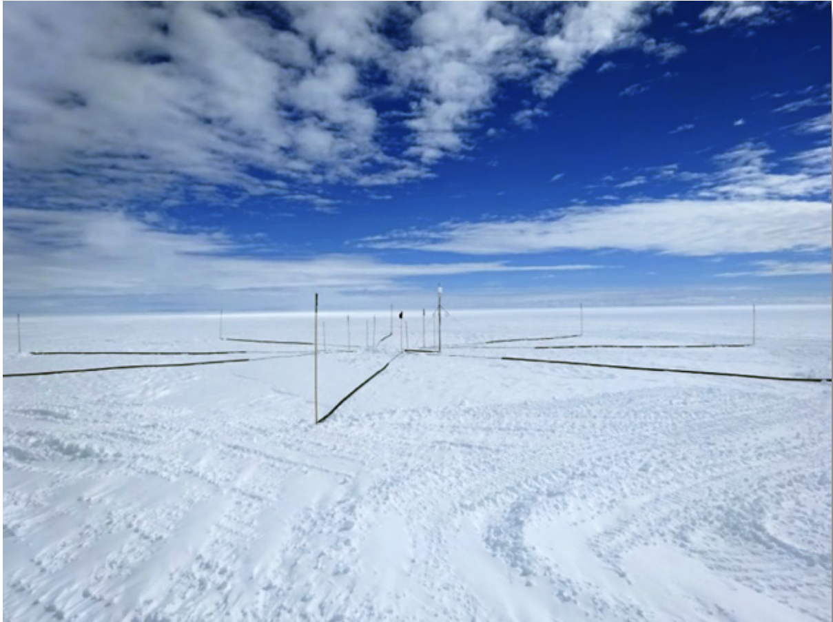
Fig. 4.4.2: One of the nine infrasound elements after recovering from snow. Flagpoles mark the outer positions of the air-pressure inlet-tubes which are part of the wind-noise-reduction-system. In the center, a field-box is buried in the snow. A WiFi-Link connects each element with the Neumayer Station.
