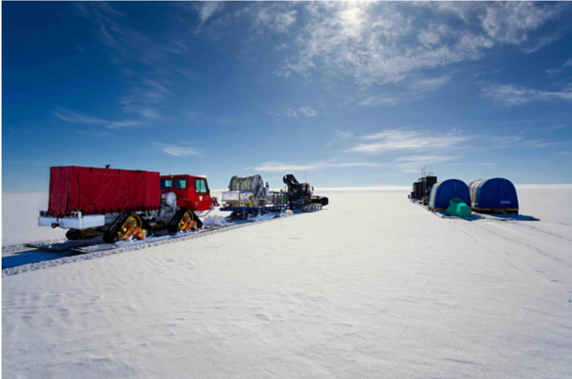
Fig. 5.2.2: The two PB trains during the traverse. On the left is the recording train with the EV, the Lehmann sled with the snowstreamer and spares and the PB. On the right we see the accommodation train with the sleeping tents and caboose (Photo: Ole Zeising).
