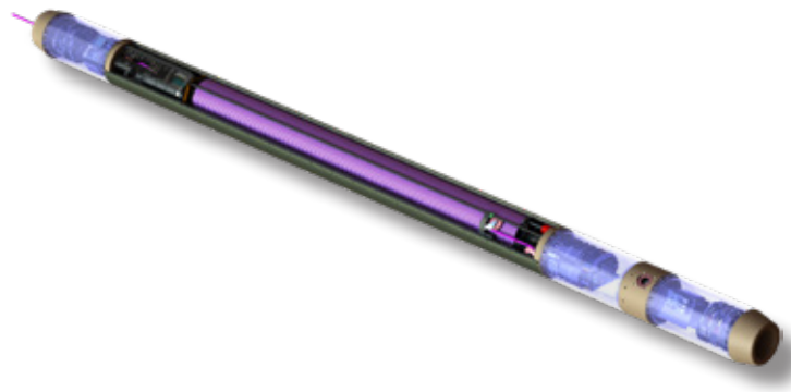
Fig. 4.26.1: Technical drawing of the modular setup of the TRIPLE-IceCraft melting probe
