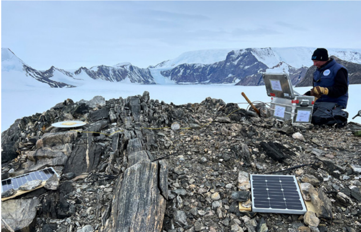
Fig. 4.25.4: Setup of GNSS campaign station STEI at Steinnabben (in the vicinity of the Swedish summer station SVEA, Heimefrontfjella).
