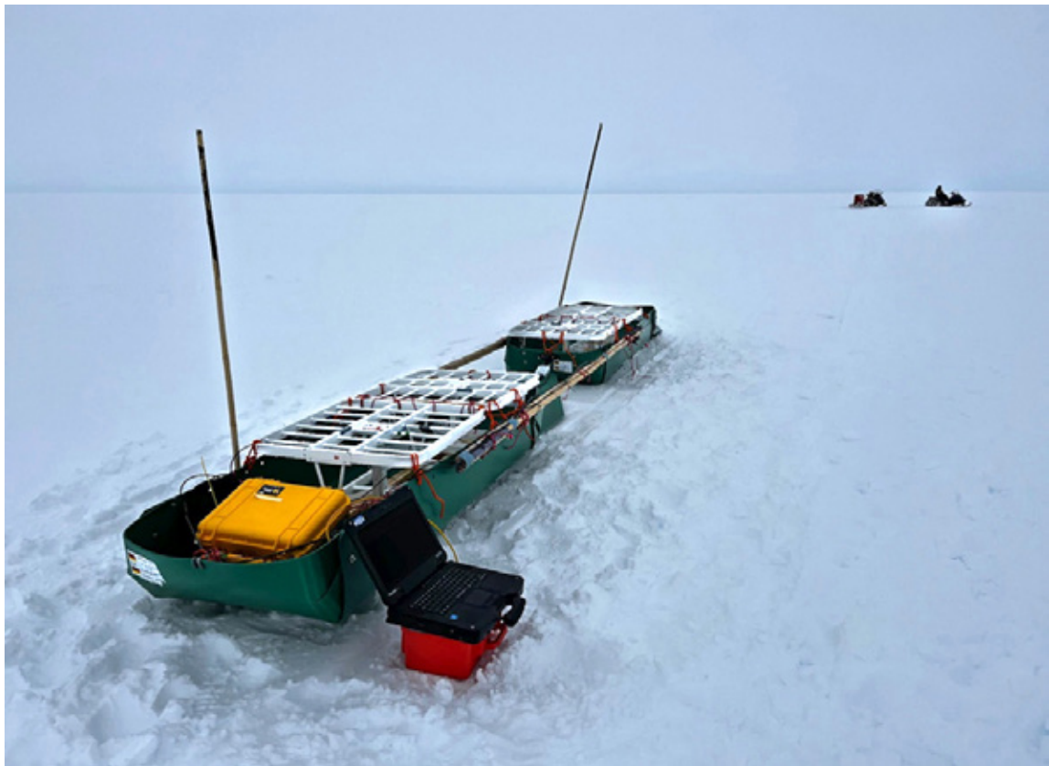
Fig. 4.15.2: Example of static data collection with a phase-coherent polarimetric radar; four antennas are used to measure the polarization dependency of the radio-wave trajectory through the ice.
