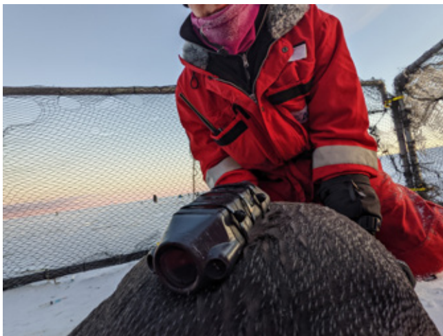
Fig.4.8.1: Deployment of a CatsCam-datalogger on an adult emperor penguin
