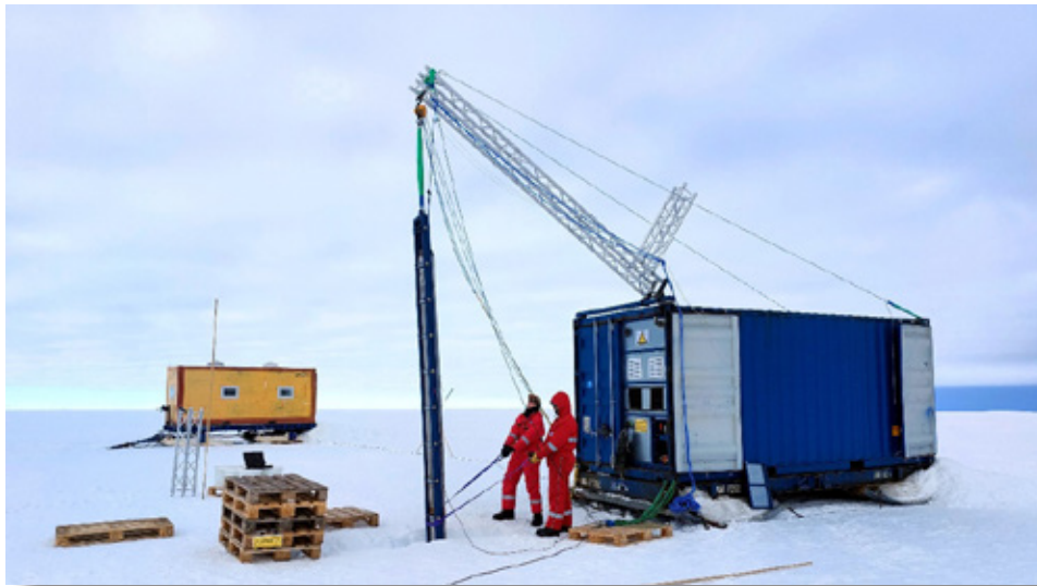
Fig. 4.26.2: Deployment of the TRIPLE-IceCraft Melting Probe
