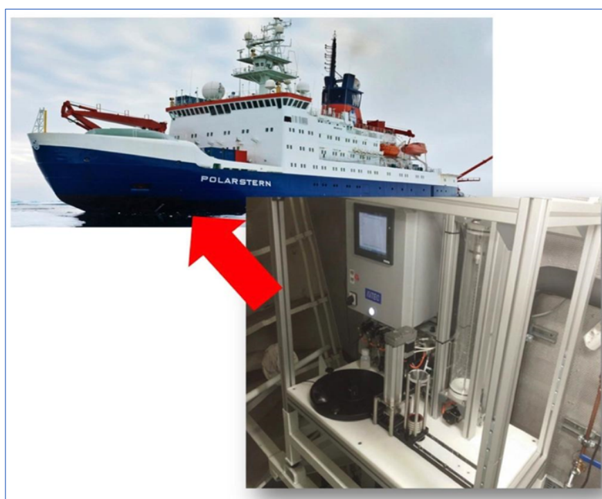
Fig. 3.3: The fully automated filtration module AUTOFIM is installed on POLARSTERN in the “Bugstrahlruderraum” close to the inflow of the ships-pump system. AUTOFIM is suitable for collecting samples with a maximum volume of 5 Liters. Filtration can be triggered on-demand or after fixed intervals.
