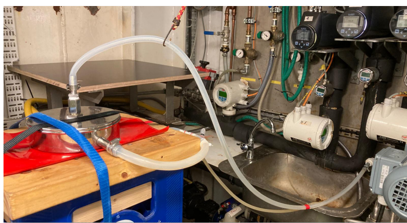
Fig. 3.1: Sieve tower ( 300 \mu\text{m} ) drawing water from the ship's "Spargel", an opening 10 m below the surface
