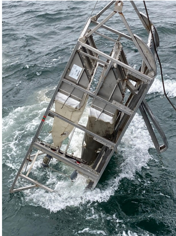
Fig. 2.3: The Epibenthic Sledge 'Berta' (Brenke 2005) hoisted back on deck after successful deployment at the Molloy Hole station PS143/1_5-4 (HG-IX)
