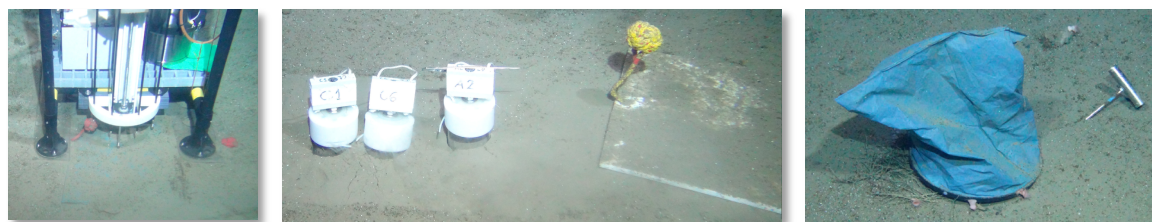
Fig. 2.12: ROV-based experiments to simulate the effects of plastic debris on seafloor communities. (Left) Microprofiler taking a measurement in the sediments covered by a plastic cover deployment. (Middle) Push cores taken after removal of the rigid plastic plate. (Right) Plastic bag covering sponge (Photos ROV-team GEOMAR, Kiel)
