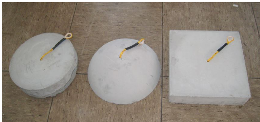
Fig. 2.8: Artificial dropstones (40x40x10 cm) of different shapes (cylindrical, spherical, rectangular)
