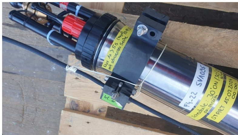
Fig. 4.7: SV1095 prior to deployment. The recorder was secured with an additional rope to the mooring line to prevent slipping.
