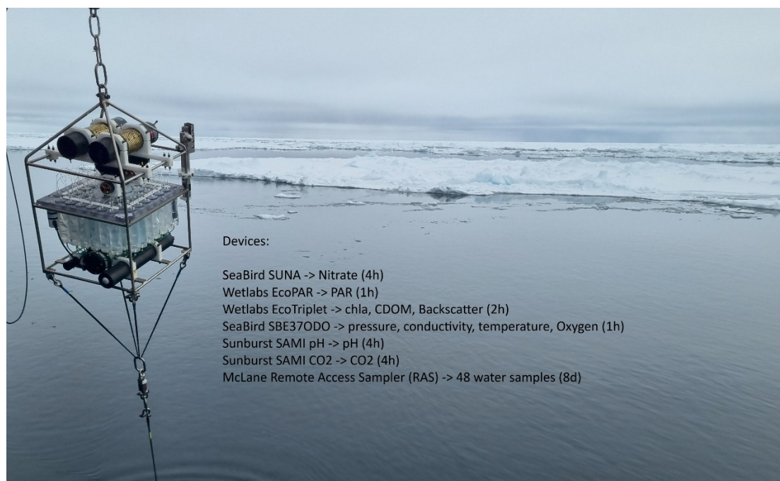
Fig. 5.5: Biogeochemical sensor package: SeaBird Suna (NO 3 ), Wetlabs Ecopar (PAR), Wetlabs EcoTriplet (CDOM, chl a , backscatter), SeaBird SBE37ODO (CTD + O 2 ), Sunburst Sami pH (pH), Sunburst Sami CO 2 (CO 2 ), McLane remote access sampler (48 water samples)
