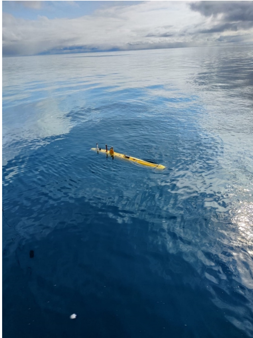
Fig 2.4: PAUL 3000, deployed during the PS148 expedition and preparing to dive
