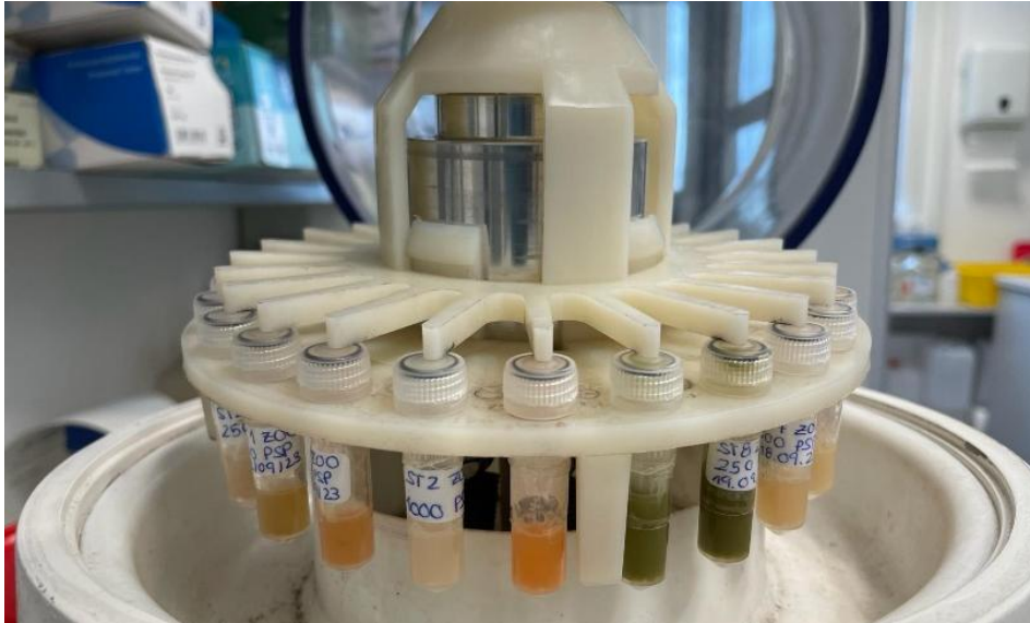
Figure 15: Zooplankton samples with Lysin beads get homogenized with the homogenizer to break the cells (Photo: Franziska Linke).
