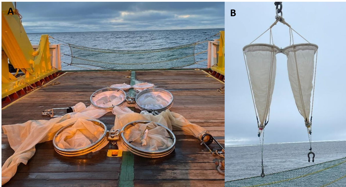
Figure 11: (A) Three plankton nets for sampling: 500 and 350 \mu\text{m} Bongo net (bottom), 150 \mu\text{m} Bongo (middle) and 20 \mu\text{m} phytoplankton net (top); (B) Phytoplankton twin net (Photos: Franziska Linke).
