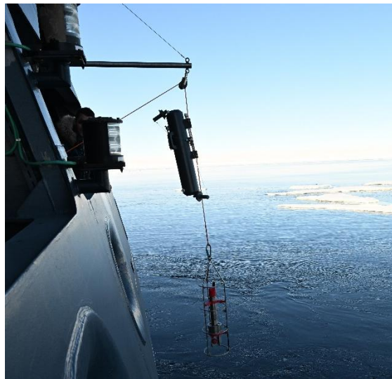
Figure 14: Sampling with the Niskin-Bottle and CTD-instrument (Photo: Marina Arregui).
