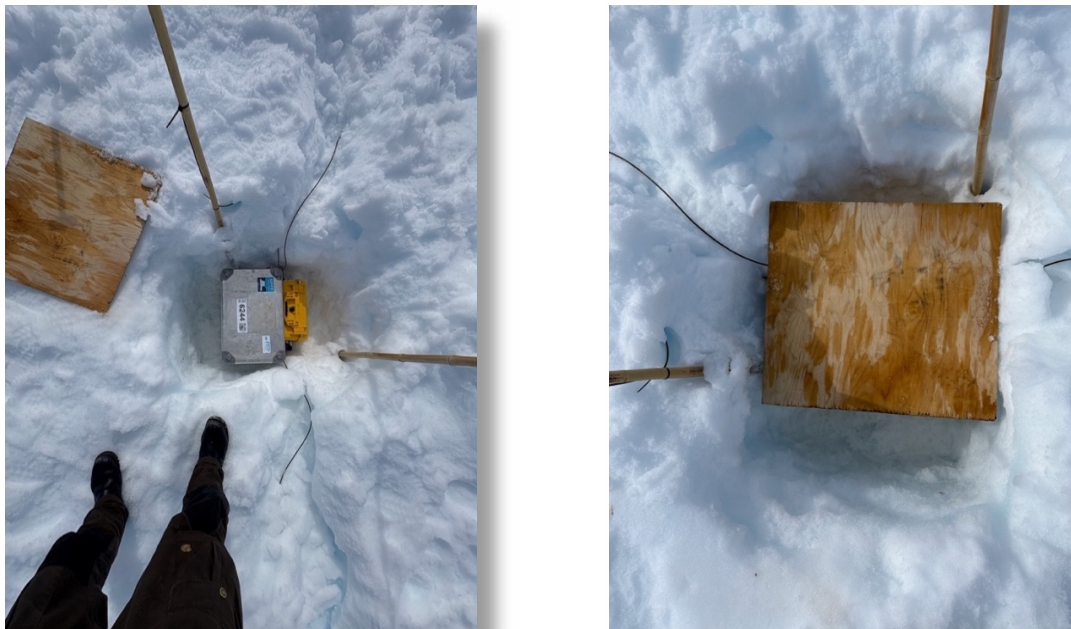
Fig.4.8.2: Left: Photograph of ApRES at station MIMO-EIS-E after maintenance on 24 January 2025 Right: Photograph of wooden sheet above ApRES at station MIMO-EIS-E
