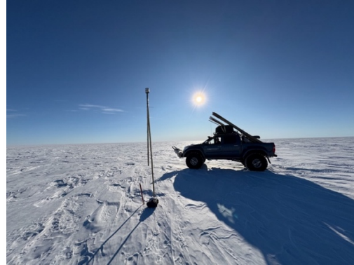
Fig. 4.8.4: Accumulation stake measurements: Left: Setup of Hilux train Right: Measuring the height of a bamboo stake higher than 2 m with an extension and a wireline device, which automatically records GPS positions.
