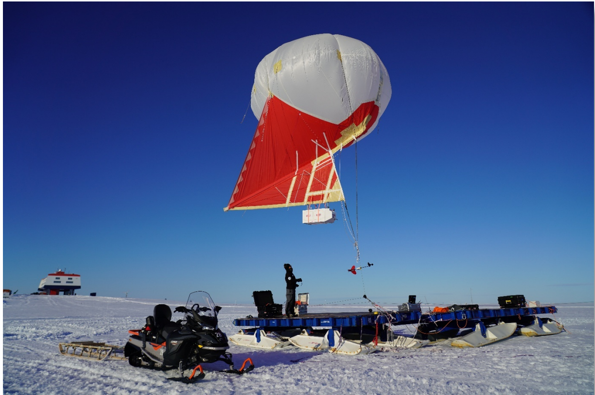
Fig. 4.19.1: Helikite take off on a clear sky day. The white payload box and the tether sonde are attached to the system. Y. Temel controls the balloon ascent speed operating one of the electrical winches fixed to the Lehman sledges. (Photo: M. Lonardi).
