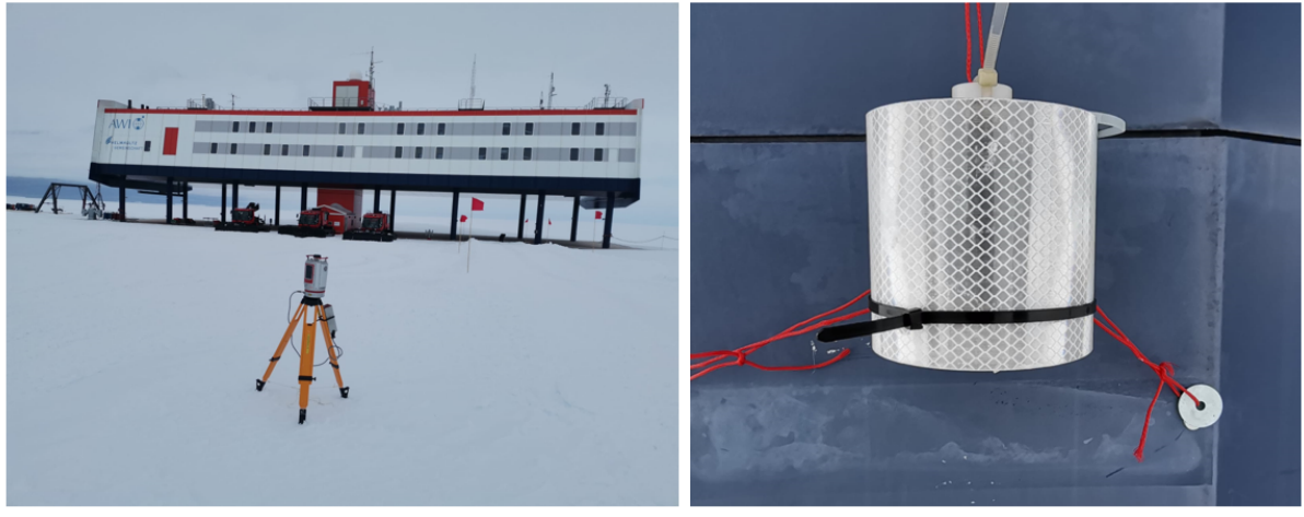
Fig. 4.17.1: Left: Terrestrial laser scanner RIEGL VZ-6000 used for the snow topography measurements around Neumayer Station III. Right: Cylinder reflector used as tie point for the local reference coordinate system of the scans.
