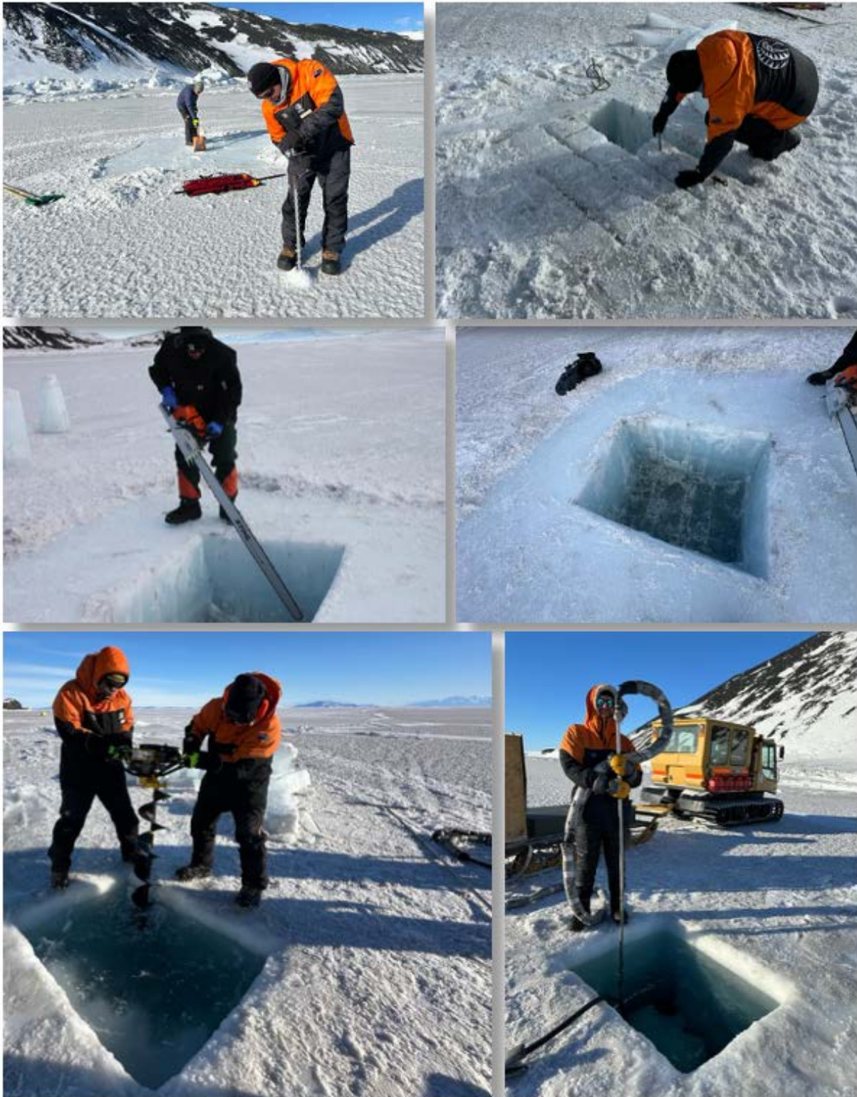
Fig. 5.5.2: The snow was removed from the ice surface and the ice thickness was determined using a Kovacs drill. A chainsaw was used to cut a rectangular opening measuring 1.7 metres by 1.2 metres into the ice, and the blocks of ice were manually removed from the ice hole. A hole was drilled through the last layer of ice with a drill so that the hole was flooded. An ice melter was used to remove the remaining ice.
