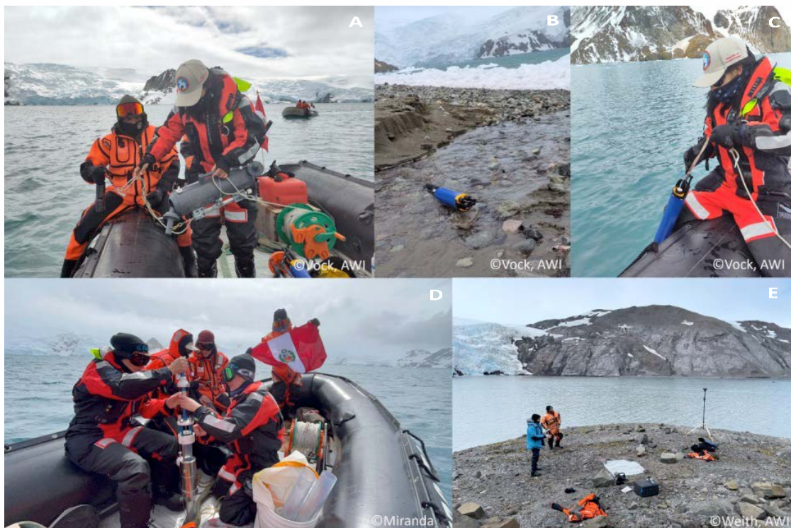
Fig. 5.4.3: ANT-Land-SIGMA-II leg 2 – impression of sampling with different gears on the coast and in the water in front of three glaciers in Admiralty Bay, King George Island, Antarctica: A) Water sampling with a Niskin bottle; B) deployment of YSI Exo 2 sonde in a meltwater stream and C) in a fjord D) Sediment sampling E) Drone missions
