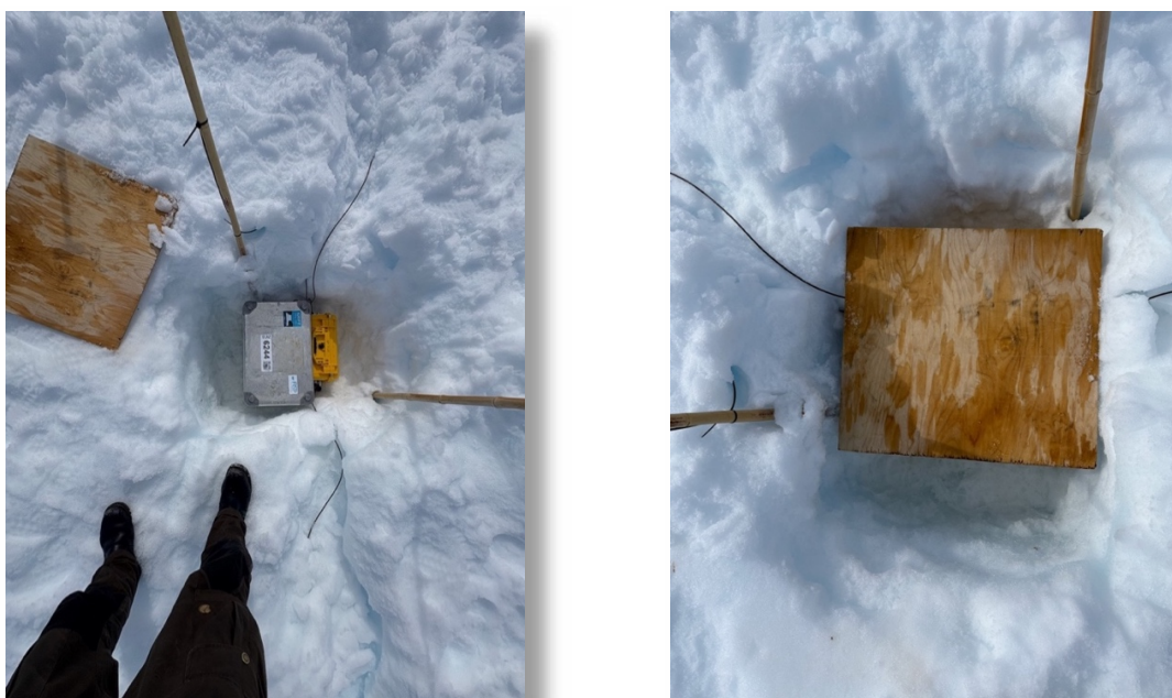
Fig.4.8.2: Left: Photograph of ApRES at station MIMO-EIS-E after maintenance on 24 January 2025 Right: Photograph of wooden sheet above ApRES at station MIMO-EIS-E
