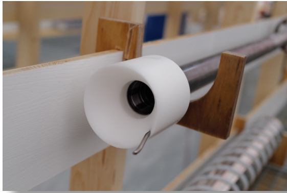
Fig. 5.1.5: Conical tool with pin mounted to outer core barrel of the rock drill. Credit: F. Wilhelms ©PNRA/IPEV
