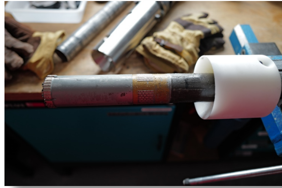
Fig. 5.1.6: The conical tool moved from the joint, the reamer and the drill head are entirely screwed into position. Credit: F. Wilhelms ©PNRA/IPEV
