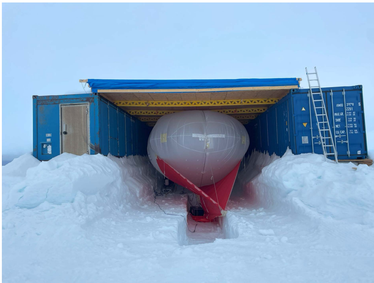
Fig. 4.19.2: The container shelter and the 64 m 3 Helikite. (Photo: Y. Temel).
