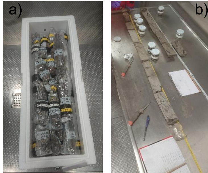
Figure 13. (a) Transported cores stored in whirlpacks and (b) cryolithological description and subsampling of BAL24-T0-UL in the climate chamber at AWI Potsdam.
