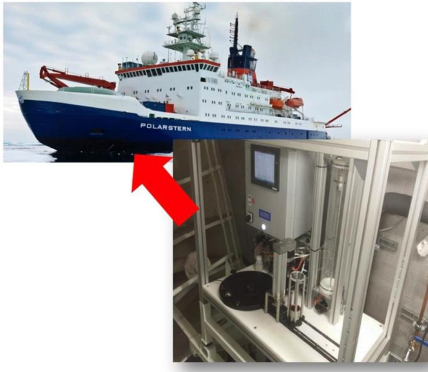
Fig. 3.1: The fully automated filtration module AUTOFIM is installed on RV Polarstern in the “Bugstrahlruderraum” close to the inflow of the ships-pump system. AUTOFIM is suitable for collecting samples with a maximum volume of 5 Liters. Filtration can be triggered on-demand or after fixed intervals. PHOTO: Katja Metfies
