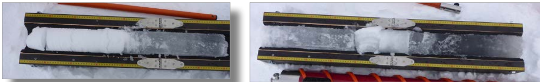
Fig. 2.7.2: Left picture: Top of core with snow; right picture: top core with snow removed + slush from coring + bottom core
