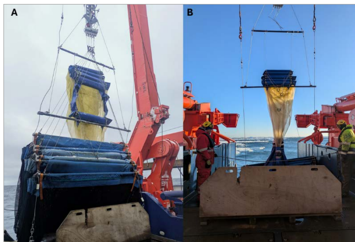
Fig. 2.2.2: mRMT set up on deployment, noting the open bottom RMT 1 net (A) and on recovery, noting all nets released and closed (B). Photos: Jennifer Freer.
