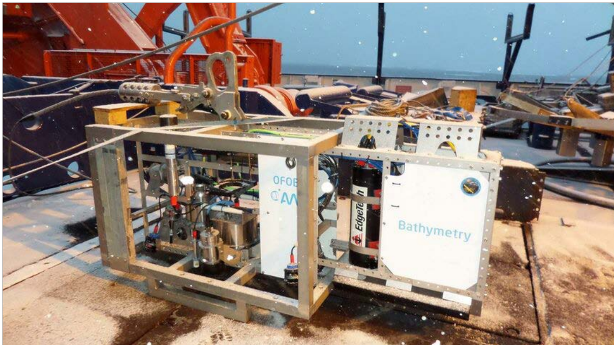
Fig. 2.3.7: The Ocean Floor Observation and Bathymetry System (OFOBS) of the Alfred Wegener Institute (Foto: Autun Purser)
