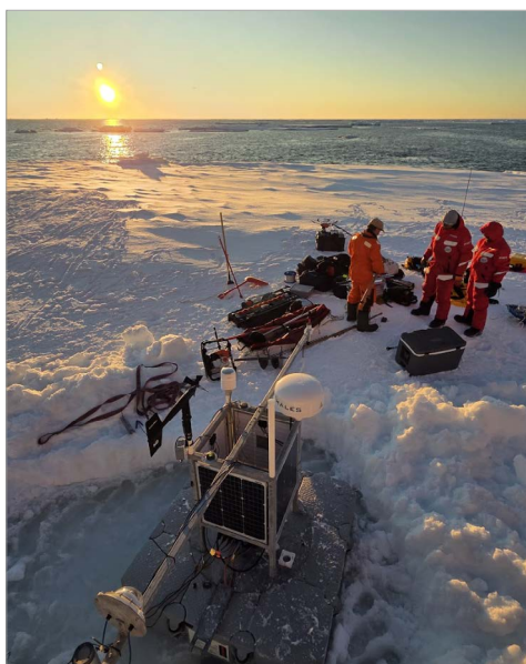
Fig. 2.7.26: 096 system deployed, before batteries and underwater sensors installation
