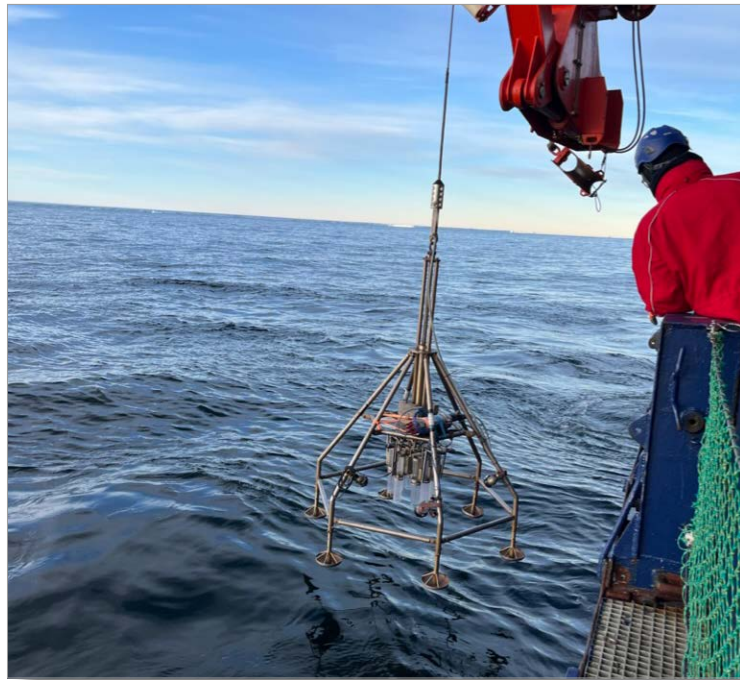
Fig. 2.3.1: TV-MUC deployed over the side of Polarstern (Foto: H. Link/ Uni Rostock)
