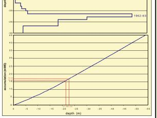
137Cs activity of drilling chips samples versus depth. The sample with the Top: highest activity includes the horizon from 1962/63 with radioactive deposition from nuclear tests in 1961/62
