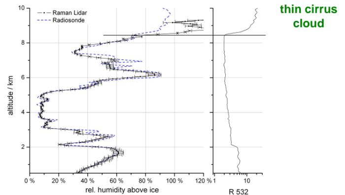
Comparison of lidar (black) and radiosonde (blue) measurements of water vapor (in terms of the relative humidity). The sonde was started at 22:45 of June 17 2003 and reached 10 km about half an hour later. The graph at the right hand side shows the backscatter ratio profile determined by the lidar at the same time (22:53 - 23:05, 20,000 shots). Up to the thin cirrus cloud in 8.5 km altitude the measurements by the radiosonde and lidar agree very well.
