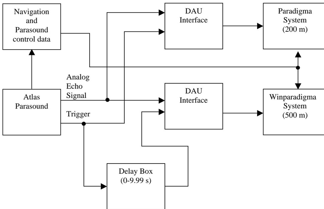
**Fig. 3.1:** Flare registration system of the SO178-KOMEX cruise.
