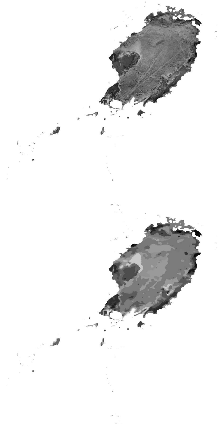
Fig. 4. Masked version of the SAR image in Fig. 3 (top), and the masked equivalent deformed ice chart for the SAR image (bottom). \hat{T}_{def} value increases from darker to lighter gray tones.
