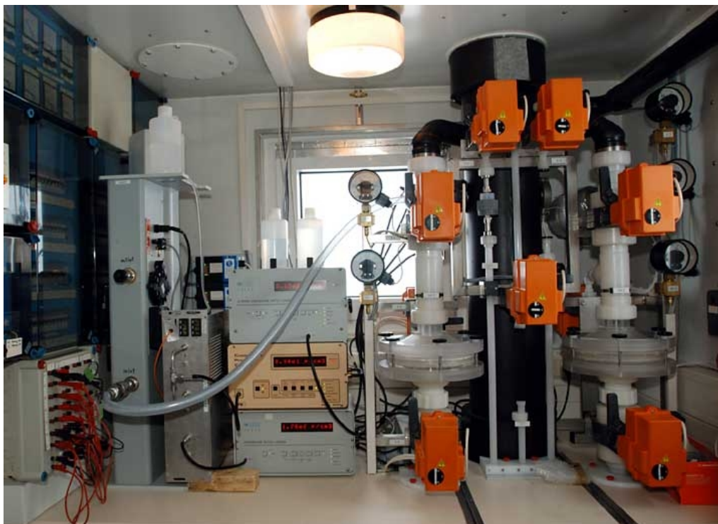
Fig. 2: A view inside the Air Chemistry Observatory: Aerosol sampling on filters (right hand), integrating nephelometer and condensation particle counters (left hand).
