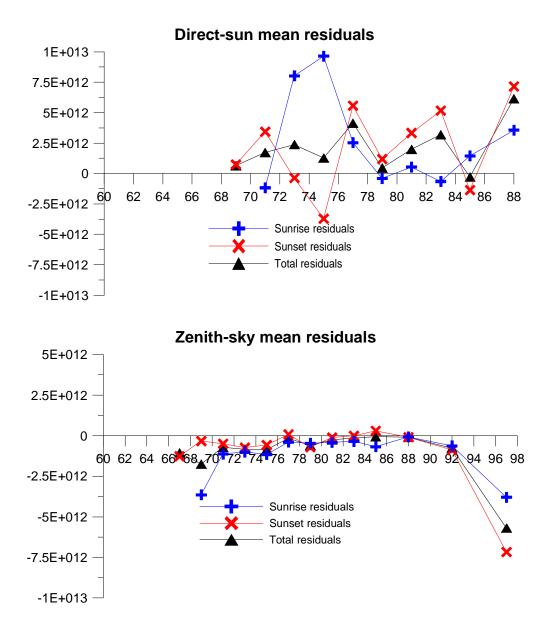
**Figure 8.6**: The mean residuals for all retrieval fits to the data. The upper plot displays the mean residuals for the direct-sun measurement fits. The lower plot displays the mean residuals for the zenith-sky measurement fits. Clear systematic errors are evident in the direct-sun fit with filter changes. The zenith-sky residuals show a systematic large residual for the highest SZA.
