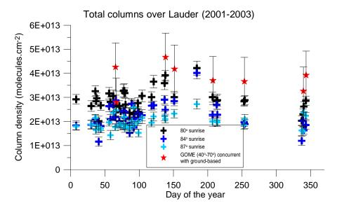
**Figure 7.7**: The total BrO columns retrieved from ground-based sunrise measurements over Lauder 2001-2003 are compared with the total columns from concurrent GOME overpasses (2001-2002).
