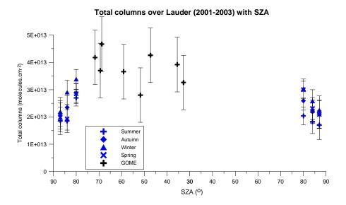
**Figure 7.8**: The variance weighted mean total columns for each season retrieved from ground-based measurements at Lauder, 2001-2003 are displayed with SZA. The concurrent GOME measurements made over the 2001-2002 period are also displayed.
