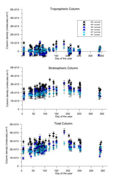
**Figure 7.3**: The retrieved tropospheric (top plot), stratospheric (middle plot) and total (lower plot) columns for BrO over Lauder 2001-2003. The retrieved columns are divided into sunrise and sunset columns for the three SZA of 80°, 84° and 87°.
