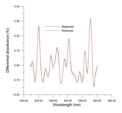
**Figure 4.6**: The spectral fit for ring at 88.1° SZA for the zenith-sky measurements made on day 254, Lauder 2001, sunset.
