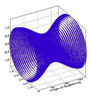
Figure 5.3: Rayleigh scattering phase function calculated for  $\lambda=350\,\mathrm{nm}$ . The highest probability for scattering is in the forward and backward directions. Scattering perpendicular to the incident light path is least likely.
