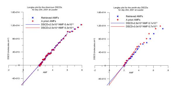
**Figure 4.7**: The Langley plot for the direct-sun DSCDs for day 254, 2001 at Lauder is displayed on the left. The Langley plot for the zenith-sky measurements is shown on the right.
