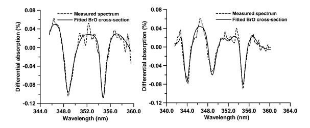
**Figure 4.4**: The typical spectral fits for BrO at 87.3° SZA for the direct-sun (left) and 88.1° SZA for the zenith-sky (right) measurements made on day 254, 2001, sunset at Lauder. The small scale features are remnants of Ring fitting procedure.
