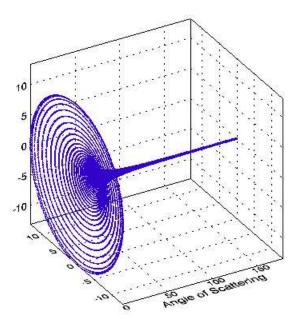
**Figure 5.4**: Mie scattering phase function, the highest probability for scattering is in the forward direction. This is calculated for aerosol particles with an effective radius of 6  $\mu$ m for 300 nm <  $\lambda$  <1200 nm.
