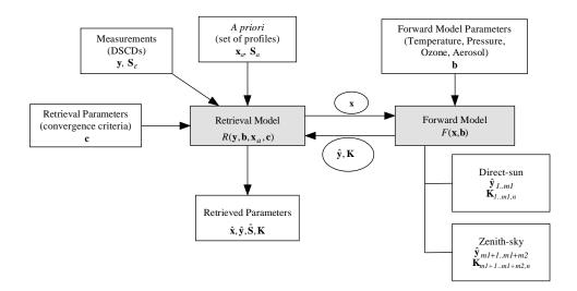
**Figure 6.1**: A schematic diagram displaying the basic structure of the retrieval algorithm. The inputs that are necessary and how the forward model and inverse models can be effectively separated is clearly shown.
