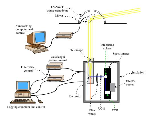
Figure 4.2: Schematic diagram of the instrument set-up for the direct-sun viewing geometry.
