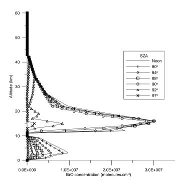
**Figure 8.4**: The stratospheric diurnal variation calculated using a Lagrangian box model (*Kreher et al.*, 2003) for sunset on day 280, 2002 at Arrival Heights, Antarctica. The polar 0° tropospheric profile is from polar balloon measurements (*Fitzenberger et al.*, 2000) and a diurnal decrease was assumed. These profiles are used as the *a priori* for the column retrievals from all measurements at Arrival Heights.
