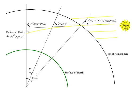
Figure 5.6: Schematic diagram illustrating how the local SZA  $(\xi)$  is determined for each path segment using the earth centric angle  $(\psi)$  associated with the path. Once  $\xi$  is obtained the correct value for concentration of the diurnally variant absorber  $N_Y(z,\xi)$  can be found.
