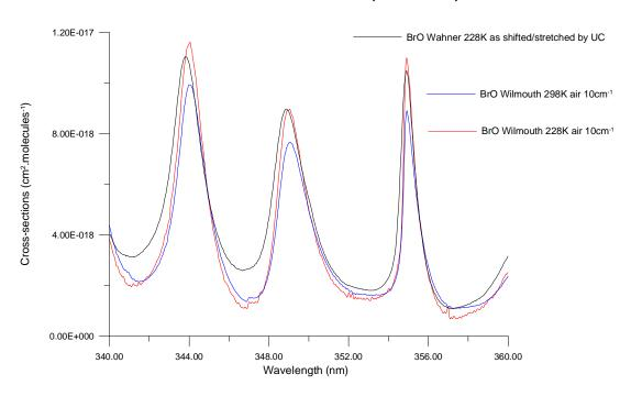
**Figure 4.5**: The cross-section for BrO from *Wahner et al.* (1988) at 228 K shifted and stretched, and the more recently measured cross-sections at 228 K and 298 K of *Wilmouth et al.* (1999).
