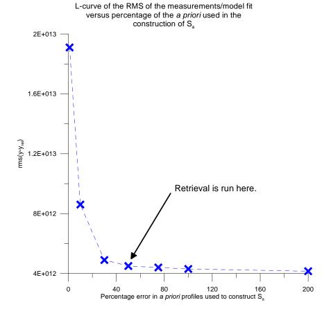
**Figure 6.2**: The L-curve for the profile retrieval from measurements made at Lauder on day 254, 2001.  $S_a$  is adjusted to ascertain a error which obtains the maximum amount of information from the measurements without mapping their errors into the retrieval.
