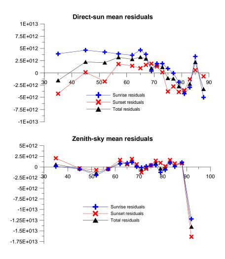
**Figure 7.6**: The mean residuals for all retrieval fits to the data. The upper plot displays the mean residuals for the direct-sun measurement fits. The lower plot displays the mean residuals for the zenith-sky measurement fits. Clear systematic errors are evident in the direct-sun fit with filter changes. The zenith-sky residuals show a systematic low residual for the highest SZA.
