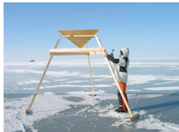
Figure 4 Corner reflector being erected on Bay of Bothnia sea ice on March 14 th 2005 (courtesy of AWI).
