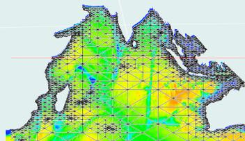
Fig. 4 Automatically generated refined mesh of Indian Ocean
