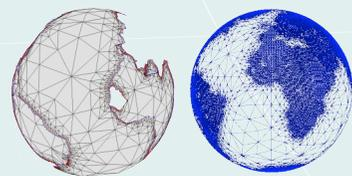
Fig. 3 Mesh of world ocean, and global mesh with refinement along topography gradients.
