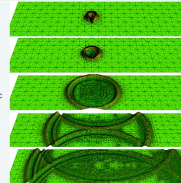
Fig. 13 Wave propagation in a prototypical tsunami model
