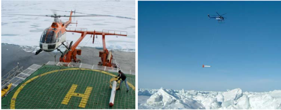
Figure 2: AWI HEM bird during take-off from the helicopter deck of an icebreaker, and during operation at 15 to 20 m above the ice surface (right photo courtesy J. Wilkinson).
