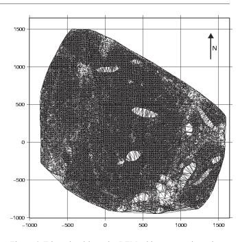
Figure 6. Triangulated irregular DEM with an approximated step size of 10 m of Samoylov Island: *x*- and *y*-coordinates are in a local coordinate-system (scale in m).
