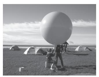
Figure 4. Tethered balloon, filled with helium, diameter 2-3 m.
