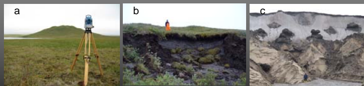
Investigation of periglacial features in the Lena Delta in summer 2008. (a) Tachymetric measurement of a pingo on Kurungnakh Island. (b) Retrogressive thaw slump on a thermokarst depression slope. (c) Typical Ice Complex deposits in the Lena Delta.
