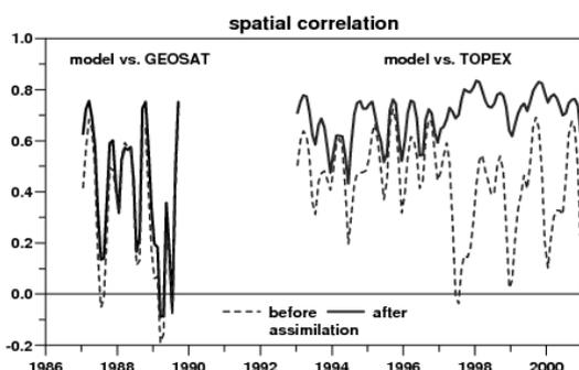
Figure 2: Spatial correlation between the sea level anomalies from the altimetric measurements and the model results without assimilation (dashed lines) and for experiment GETO20.
