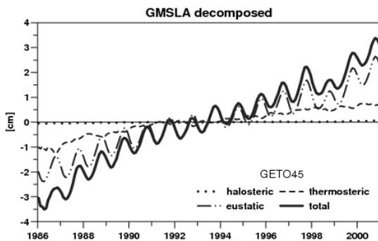
Figure 5: Global mean sea level anomaly (GMSLA) from experiment GETO45 (thick line) broken down to the halosteric (dotted), thermosteric (dashed) and eustatic (dash-dotted) contribution.
