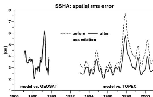
Figure 3: Root mean square error (RMS) between the sea level anomalies from the altimetric measurements and the model results without assimilation (dashed lines) and for experiment GETO20.
