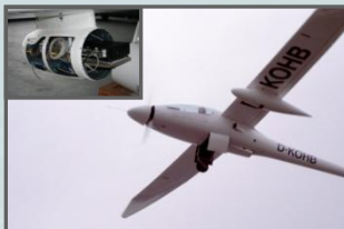
Fig. 2: Motor glider with hyperspectral sensor and equipment in the wingpod (Photo: OHB).
