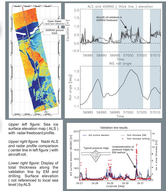
Upper left figure: Sea ice surface elevation map (ALS) with radar freeboard profile.
