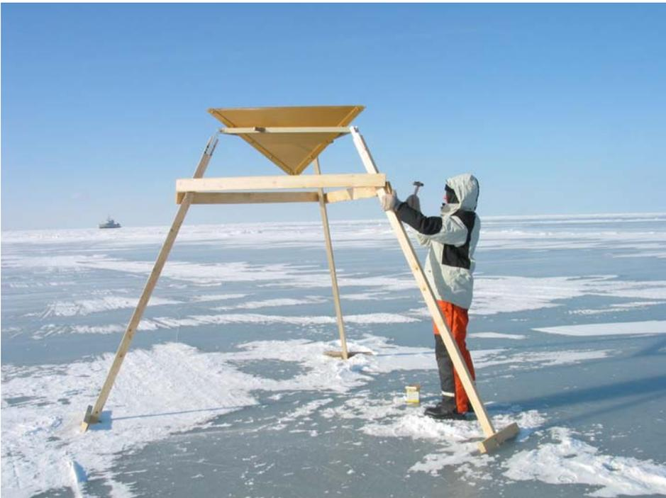
Figure 6.2-9: Picture of a corner reflector deployment site (east reflector)
