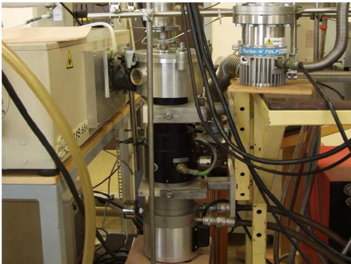
**Fig.25:** View of the cold head of the cryostat (*middle*) attached to the FTIR-spectrometer (*left*)
