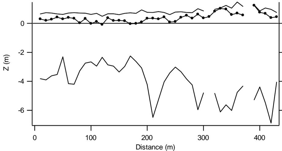
Figure 11: Drill-hole ice thickness profile along MYI validation line between southern (at  $x = 0$  m) and northern (at  $x = 430$  m). From top to bottom, surface elevation, freeboard, and draft are shown.  $Z = 0$  m indicates the vertical location of the water level.
