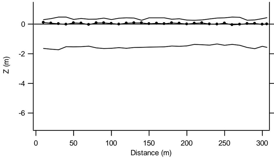
Figure 7: Drill-hole ice thickness profile along FYI validation line between eastern (at  $x = 0$  m) and western (at  $x = 306$  m). From top to bottom, surface elevation, freeboard, and draft are shown.  $Z = 0$  m indicates the vertical location of the water level.
