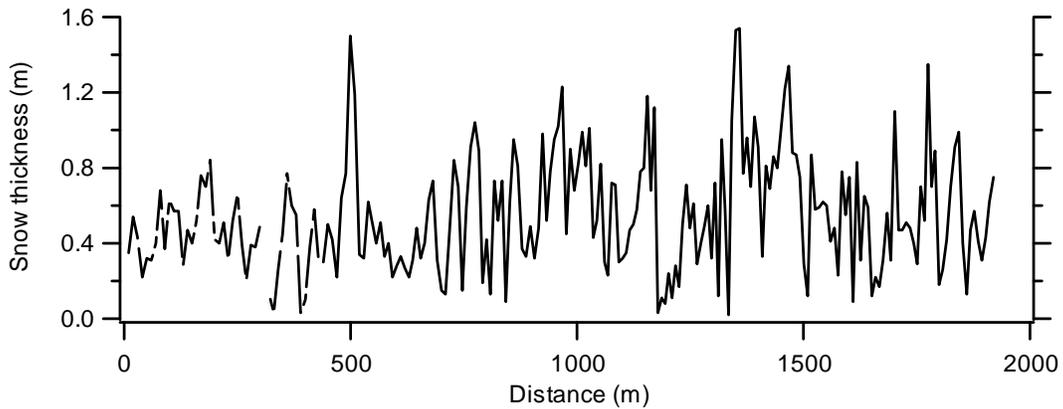
Figure 13: Snow thickness profile on the multiyear site. Stippled line shows measurements along main validation line (cf. Fig. 11), and solid line extends north from the northern corner reflector at  $x=0$  m, in the same direction as the main line and aircraft surveys.
