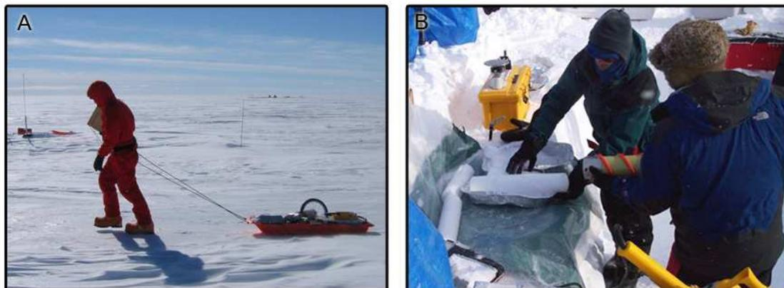
Figure 1.3.: Ground-based activities during CryoVex 2004. (A) The man-pulled sledge hosting GPR and GPS-systems. (B) Retrieval of a shallow firn-core for physical properties measurements.
