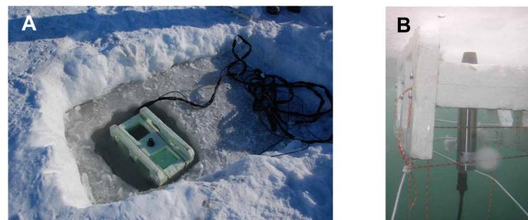
**Figure 2:** (a) Sensor mounted on under-ice sled for transmittance measurements (b) under-ice sensor in operation.
