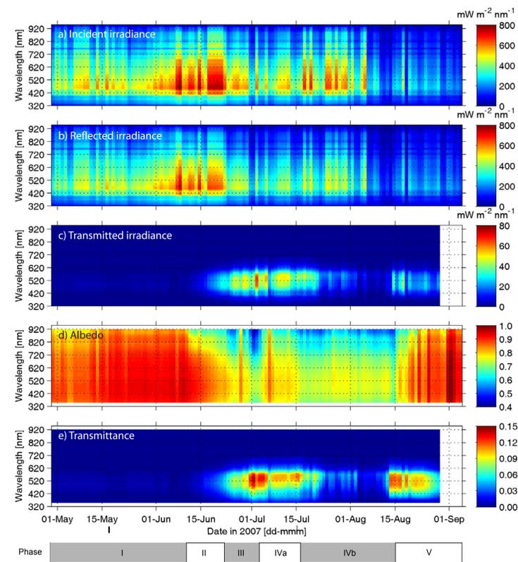
**Figure 3:** Time series (one spectrum per day) of (a) incoming, (b) reflected, and (c) transmitted spectral irradiance, (d) spectral albedo, and (e) spectral transmittance measured in the Central Arctic at Tara 2007 (from Nicolaus et al., 2010b). As the under-ice sensor had to be retrieved on 28 Aug., no transmitted data are available afterwards.
