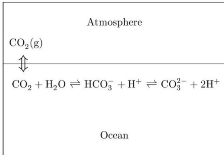
Figure 1.1.1: Schematic illustration of the carbonate system in the ocean. CO<sub>2</sub> is exchanged between atmosphere and ocean via equilibration of CO<sub>2</sub>(g) and dissolved CO<sub>2</sub>. Dissolved CO<sub>2</sub> is part of the carbonate system in seawater that includes bicarbonate, HCO<sub>3</sub><sup>-</sup>, and carbonate ion, CO<sub>3</sub><sup>2-</sup>.
