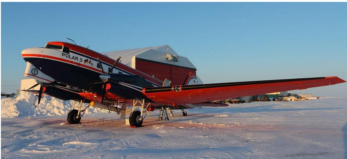
**Figure 2.1.:** Polar-5 in Barrow during SIZONet 2011. The EM-Bird can be seen below the aircraft body.
