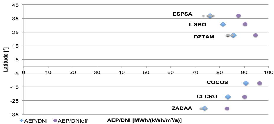
**Figure 6: Variation of ratios AEP/DNI and AEP/DNI<sub>effective</sub> with changing latitude.**
