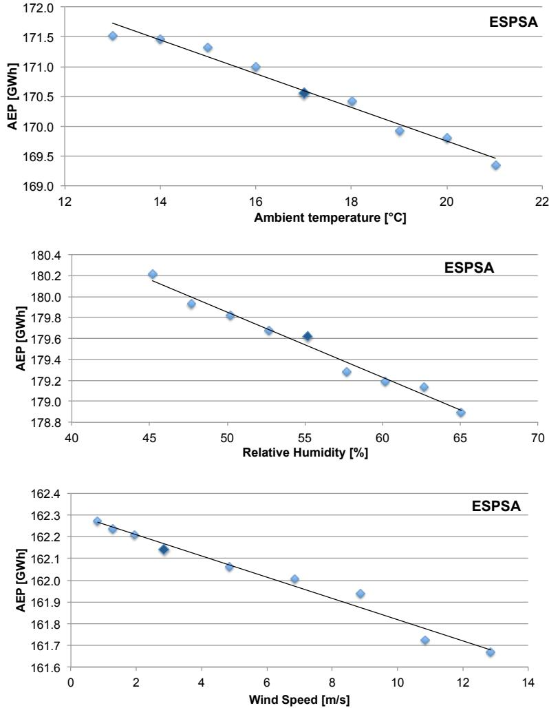
**Figure 7: The variation of AEP at site ESPSA for PT with change in meteorological parameters. Top: With increase in ambient temperature, AEP decreases. Middle: As relative humidity increases, AEP decreases. Bottom: Wind speed increase results in decrease in AEP. Large markers represent reference case**
