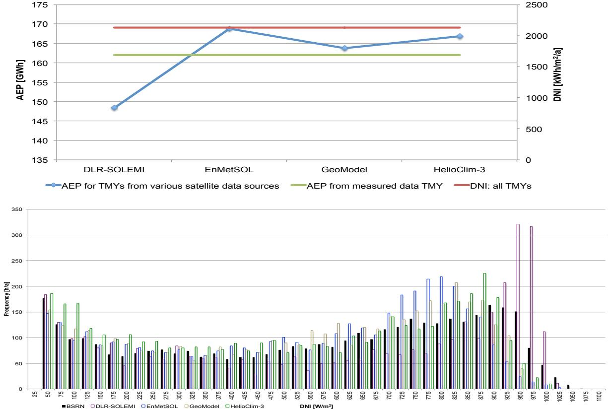
**Figure 3: Top:** Figure comparing AEP from TMYs created from different data sources for site ESPSA. The green line represents reference AEP from ground-measured TMY. DNI values are almost same for all TMYs. **Bottom:** Comparison of DNI frequency distributions of TMYs created from different sources with that from ground-measured TMY at site ESPSA. The black bars represent frequency distribution from ground-measured TMY.
