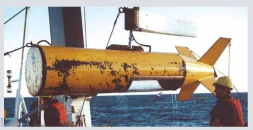
Deploying a deep acoustic towbody from the research vessel Tangaroa to survey deep-sea fish stocks off New Zealand. Acoustic surveys are regularly carried out to monitor the size of spawning aggregations of species such as orange roughy and oreo dories.
