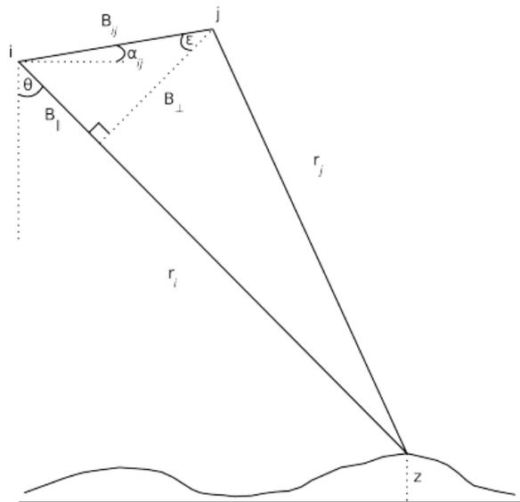
Figure: Setup for interferometric imaging.
