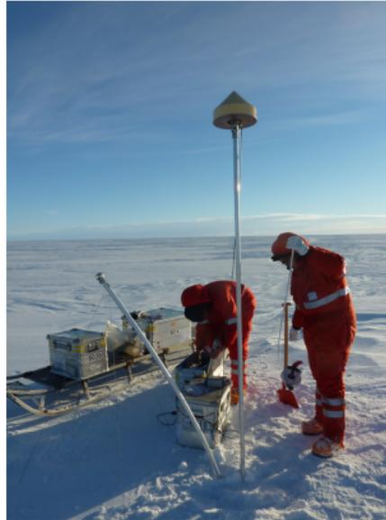
**Figure:** Ground Penetrating Radar and Global Positioning System measurements (LIMPICS ANT-Land campaign 2009/2010).
