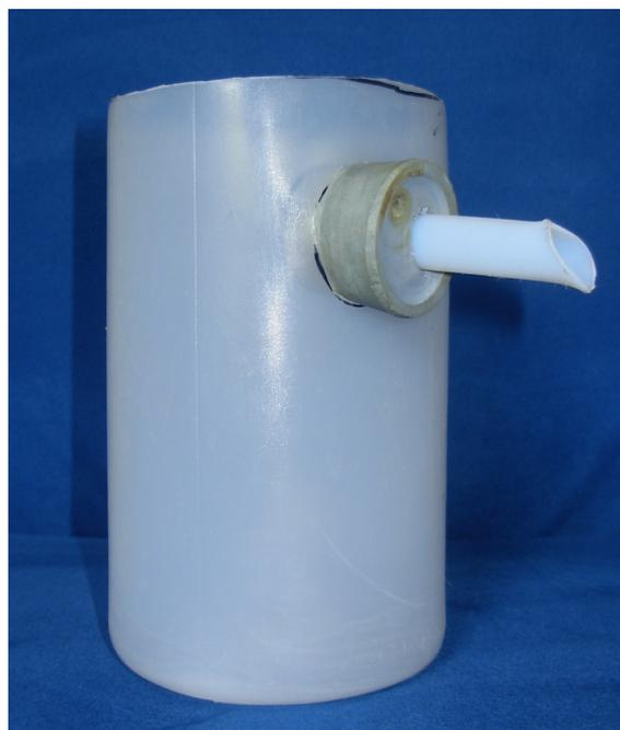
Fig. 13: Overflow-cylinder as equipment for density measurement (Photo: K. Fröb 2011).
