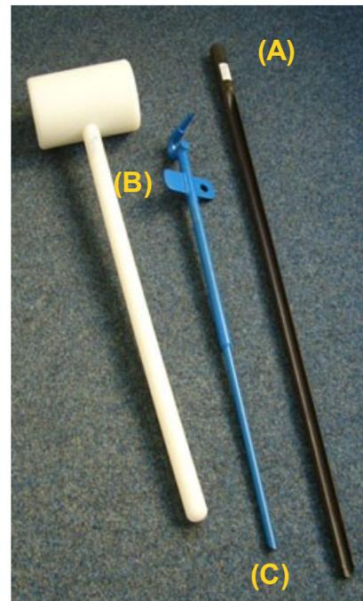
Fig. 8: Pürckhauer drill (A); sledge (B) and lever (C) (source: ECO TECH).
