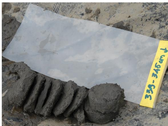
Fig. 10: Sample bag with sample and note of depth and direction of core (Photo: J. Boike 2009).
