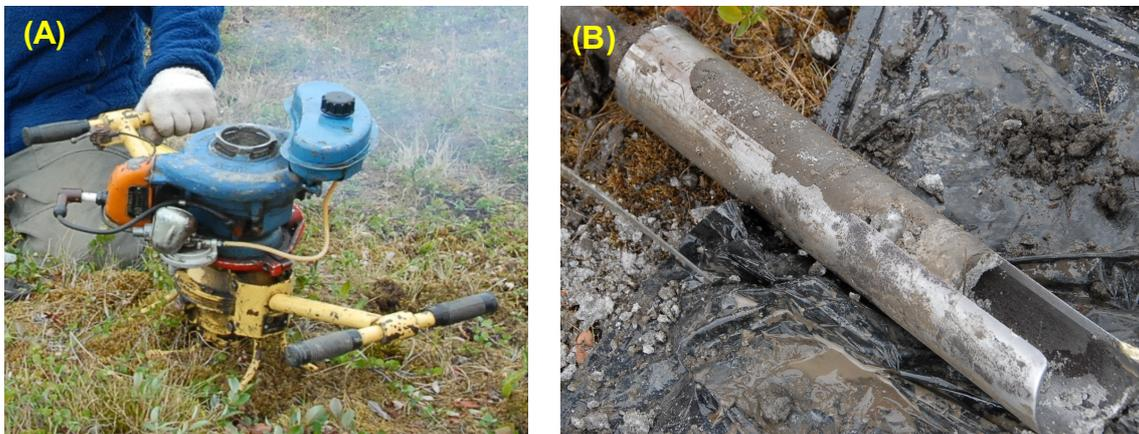
Fig. 9: Drilling equipment: (A) engine for penetrating the ground, (B) drilling head with sample (Photo: J. Boike 2009).
