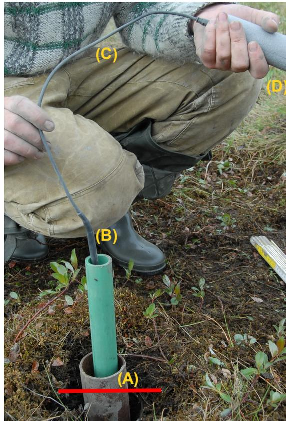
Fig. 11: Installing of temperature chain with (A) plastic tubes, (B) temperature sensor, (C) temperature chain and (D) the data logger; the red line marks the ground surface (Photo: J. Boike 2009).
