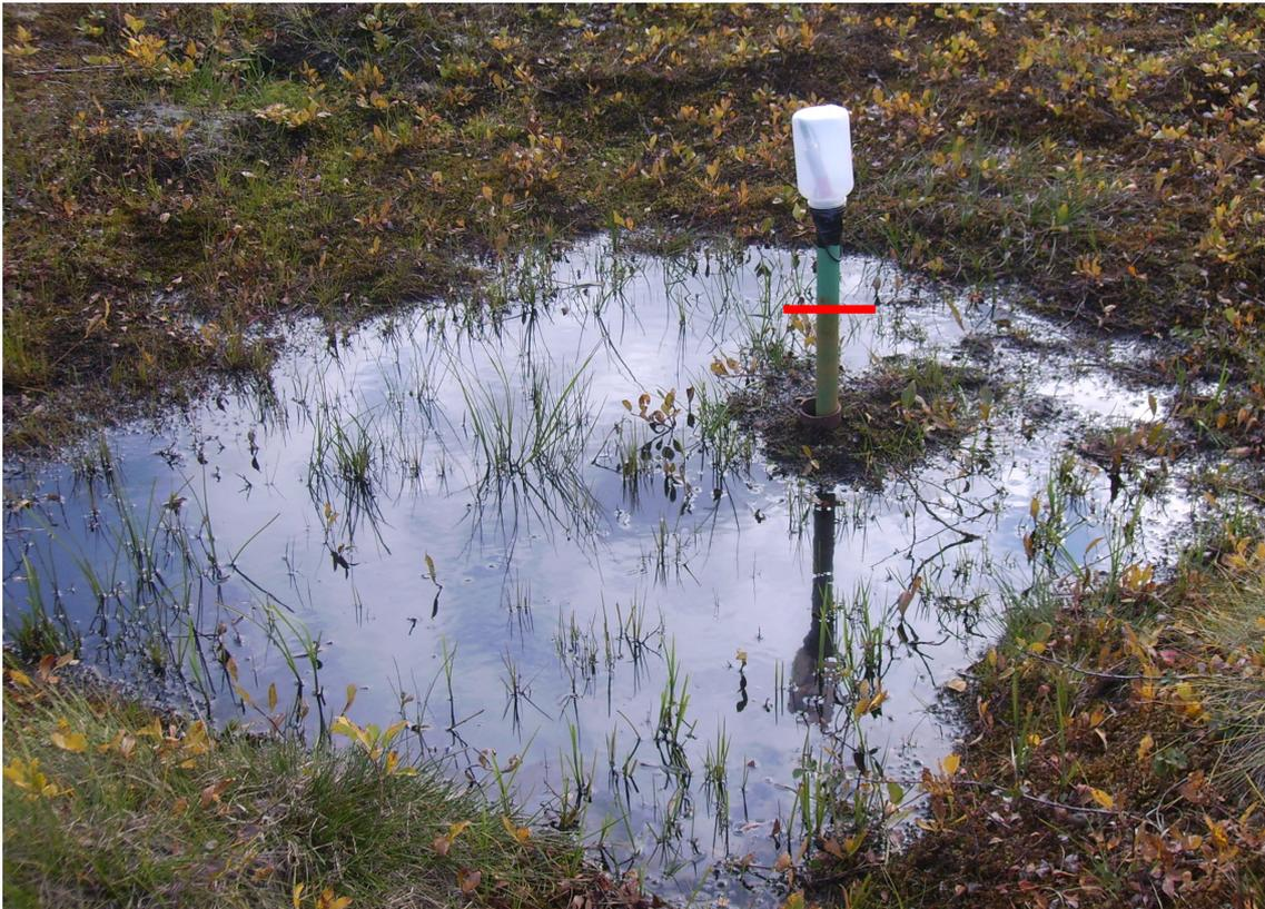
Fig. 12: Surrounding of the bore hole on Kurungnakh one year after installing the temperature chain; the red line marks the former grounds surface (Photo: M. Langer 2010).
