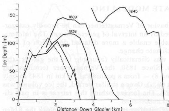
Fig. 8: Measured ice depth profiles for various years including an 1845 trimline estimate from the map of Finsterwalder (1897) and two profiles for 1969: for the specific flowline in fig. 1 (dashed), and a mean of number of flowlines (solid)
