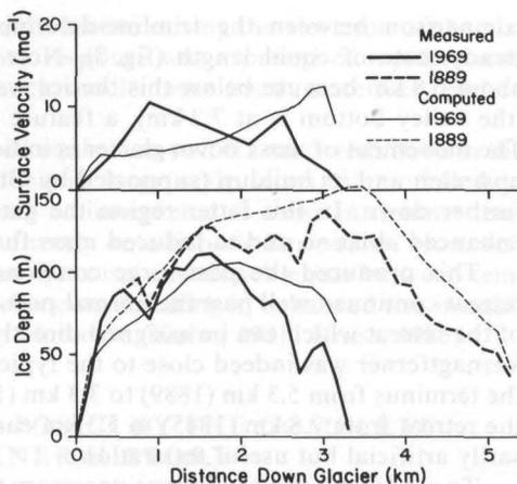
Fig. 6: Surface velocity and ice depth profiles both measured and steady state (calculated for smoothed bed using best-fit  $s$ ,  $m$  and  $C_v$  values)
