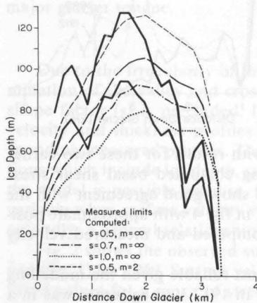
Fig 5: Steady state ice depth profiles calculated (using the smoothed bedrock of fig. 2) for a range of valley cross-section shapes ( $m = \infty$  or 2 indicates a rectangular or parabolic valley) and stress factor  $s$  values. The measured ice depth is indicated by an envelope defining the  $\pm 15\%$  error range
