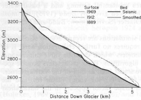
Fig. 2: Surveyed ice surface profiles down the central line of fig. 1 along with the corresponding bedrock determined directly below the 1969 terminus and by a seismic study on the glacier. The computationally more acceptable smoothed bedrock is also included
