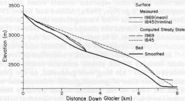
Fig. 7: Measured and modelled steady state ice surface elevation profiles for 1845 and 1969. This latter is a mean for a number of flowlines. Note that the bedrock below 7.2 km does not reflect reality, the Rofen Valley wall rising from this point
