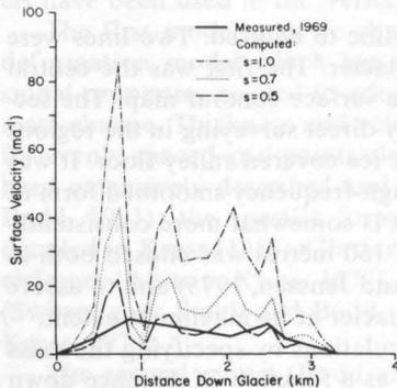
Fig. 3: Surface velocity profiles (along the central line of fig. 1) calculated for a range of stress shape factor  $s$  values, and corresponding measured velocity data
