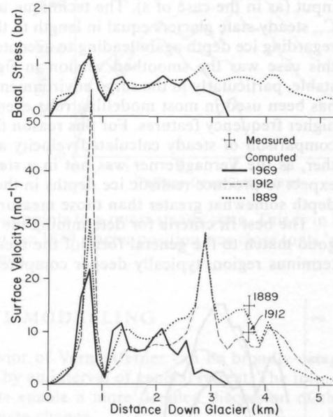
Fig. 4: Surface velocities and basal shear stresses calculated for different years from the bed and surface elevation data of fig. 2 using the best-fit  $s$  value. Single point velocity values for 1889 and 1912 are represented by magnitude and position uncertainty crosses
