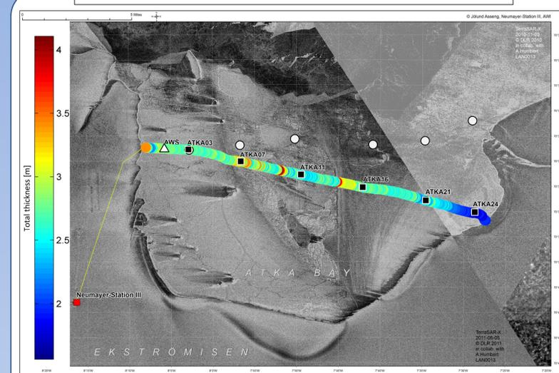
TerraSAR-X image of Atka Bay with stations in 2010 (white) and 2011 (black), where regular **manual thickness measurements** take place. Station names (e.g. ATKA03) refer to the distance to the western ice-shelf edge. The profile was relocated in 2011 in order to reduce the likelihood of an early ice break-up at ATKA07 as in 2010.
