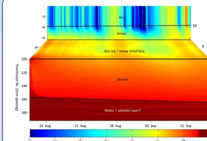
Temperatures measured by a thermistor chain deployed between ATKA03 and the ice-shelf edge. Due to technical problems, data is only available between 10 August and 15 September 2011. Air/snow, snow/ice and ice/water interfaces are visible around 50 cm, 0 cm and -120 cm. Below the solid sea ice, a layer of ice platelets might be recognizable.
