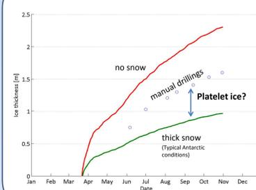
A simple Freezing-Degree-Day model was applied to compare sea-ice thickness as it would result from pure thermodynamic growth with thickness measured in the field (including platelet ice contribution) in 2011.
