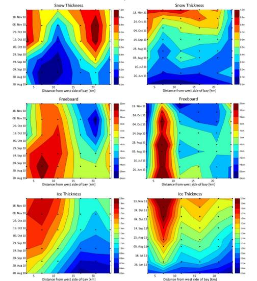
**Top:** Hovmöller diagrams of snow and ice thicknesses and freeboard across Atka Bay (Hoppmann et al., 2011). Note the different time (y-) axes in 2010 and 2011.
