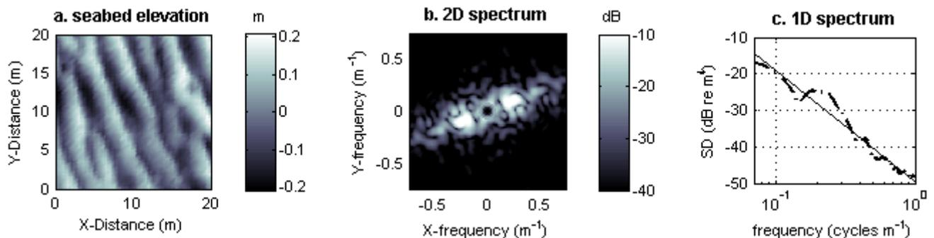
Figure 2. a. Box of seabed elevations (relative to the box mean seabed elevation) taken from the whole dataset; b. associated 2D spectrum showing the peak (mirrored) associated with the bedforms and c. 1D spectrum (dotted line) calculated by averaging the Spectral Density (SD) of the slices taken through the 2D spectrum and power-law fitted to the 1D spectrum (solid line).
