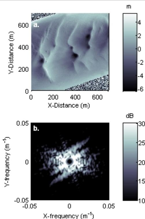
Figure 5. a. Box of seabed elevation (700 m x 700 m) taken from the whole dataset (areas without bathymetric data are padded with random values which are not 'seen' by the spectral analysis) and b. associated 2D spectrum.
