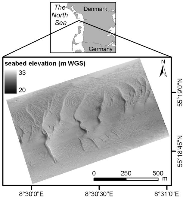
Figure 1. Location of the test area and detailed bathymetry (m WGS84). Mean sea level is equivalent to 39.39 m WGS84.
