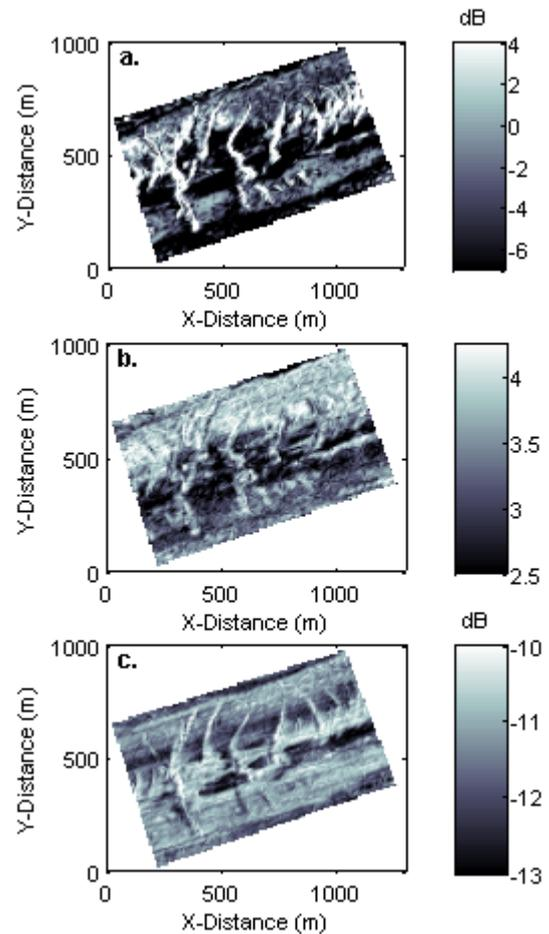
Figure 3. a. Energy of the main peak of the spectrum in each box (20 m side); b. spectral exponent and c. spectral strength (logarithmic form) of the power-law applied on the average of the slices taken through the 2D spectrum of each box.
