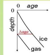
Fig. 1  $\Delta$ age: age difference between gas kept in air bubbles and surrounding ice
