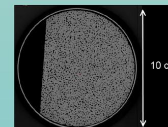
Fig. 7 Horizontal section of reconstructed firn core B22. Lighter parts show ice matrix and the sample tube, darker parts show air
