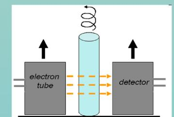
Fig. 8 schematic illustration of ice core computer tomograph
