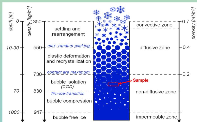
Fig. 4 Process of firn densification (modified after Blunier and Schwander)
