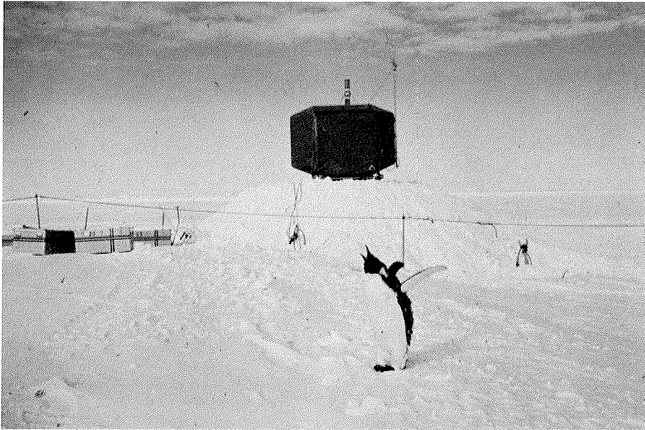
Figure 6: The trace substance observatory with meteorological sensors on the mast of the right hand side and the heated stack in the middle of the container
