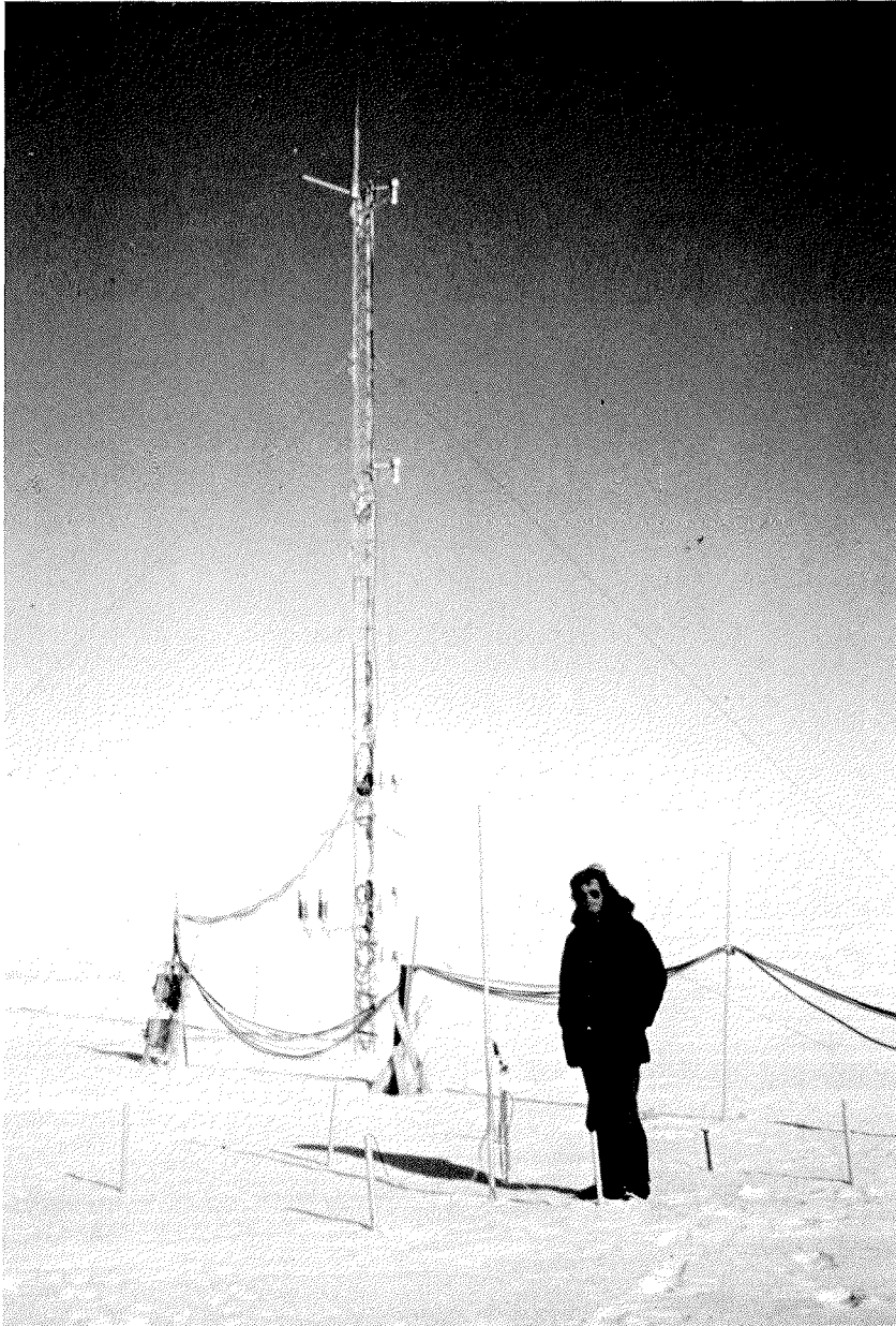
Figure 3: The small meteorological mast (height: 15 m) equipped with psychrometers
