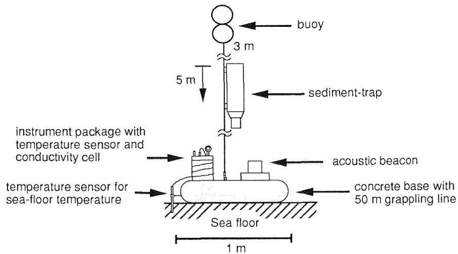
Fig. 62: Diagram of the deployed mooring in the Laptev Sea
