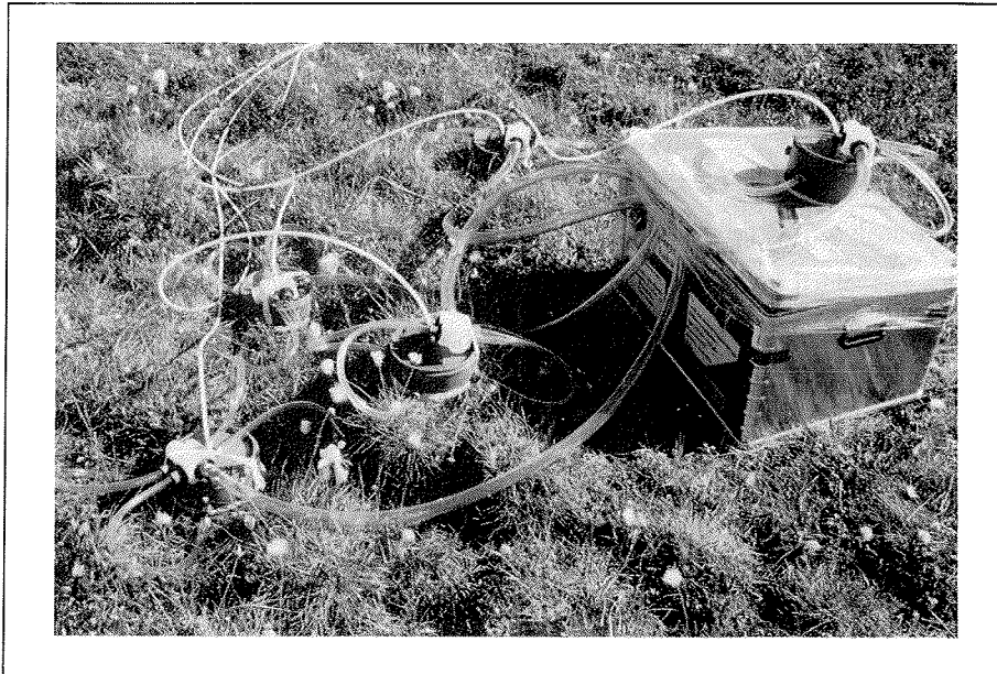
Fig. 3.2. The setup for the measurements of soil respiration in the field (tussock tundra). Chambers (red-brown), distributor containers (white, on top of the chambers), reference chamber on top of the transport box, which served as buffer volume.
