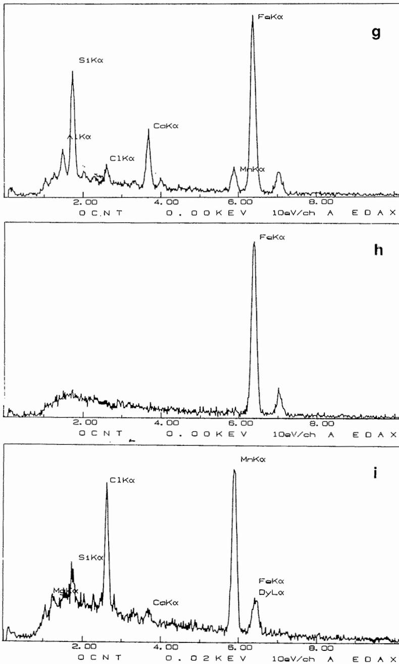
Fig. 3 (cont'd). Spectrograms of X-ray microprobe EDAX analysis.
