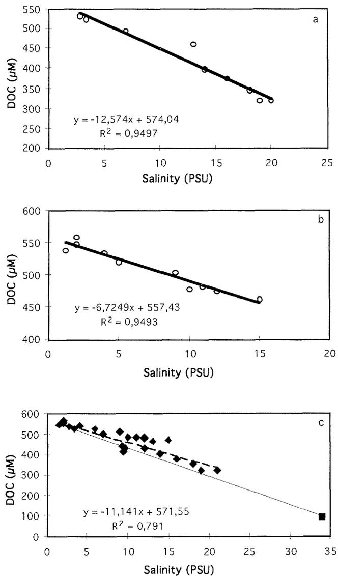
Fig. 2. Distribution of dissolved organic carbon (DOC) across a salinity gradient in the Ob (a) and the Yenisei (b) with regression line and equation showing. Panel c shows the pooled data for both rivers including intermediate stations. The broken line indicates the regression through all data points (diamonds) and the solid line indicates the conservative mixing line assuming a marine endmember DOC concentration of  $93 \mu\text{M C}$  as explained in the text.
