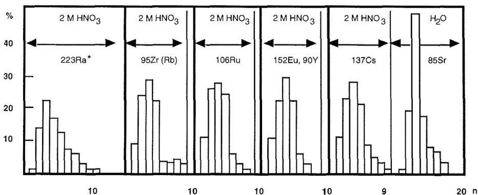
Fig. 1. Elution of interfering radionuclides through the extraction chromatographic column with tvex-DCH<sub>18</sub>C<sub>6</sub>; n - number of collectors, volume of collector is equal to 3 ml.
