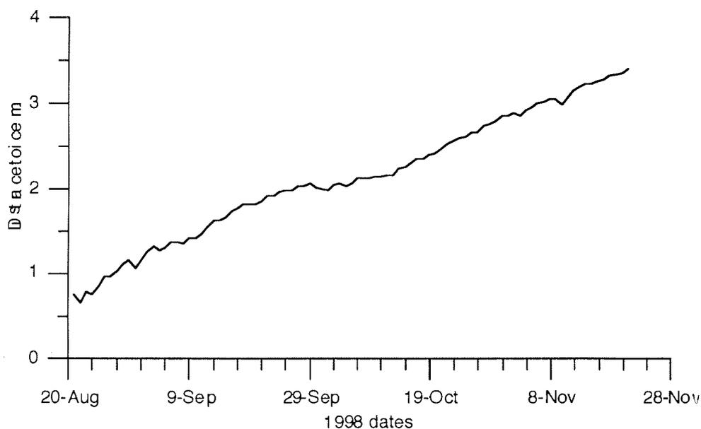
Fig. 47: Graph of echo-soundings (raw data) from beneath 79Fiord-glacier. Sounder directed upwards towards the bottom of the floating glacier tongue.
