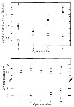
Figure I-4 Precision and accuracy of microoptodes. Precision is given as mean deviation from true oxygen saturation value [% air saturation] for water of 0% (open symbols) and 100% air saturation (filled symbols) for each of the four optodes used during our experiments (n=130 for each sensor and saturation level). Accuracy can be inferred from error bars (± 1SE). Were error bars are missing they are inside the symbol.
