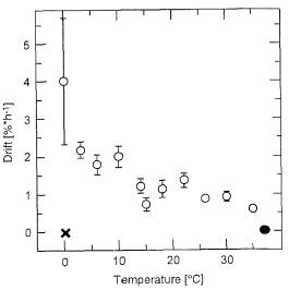
Figure I-9 Drift of oxygen sensors. Data shown are means  $\pm$  1SE for two or three sensors used in up to 36 calibration procedures (each lasting for 20-30 minutes). Circles: POS (polarographic oxygen sensors) unpubl. data O Heilmayer and M Langenbuch, AWI, dot: POS, Baumgårtl and Lübbers (1983), x: microoptodes, maximum drift in our experiments).
